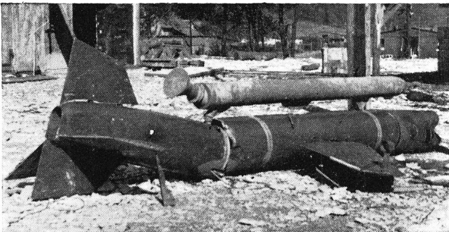
THE BUTTERFLY: Designed by Prof. Wagner of Junkers, this radio-guided anti-aircraft rocket projectile is said to exceed 600 m.p.h., have a ceiling of 50,000ft. and a range of 20 miles. It is known as the Schmetterling (Butterfly) and was about ready to go into mass production.
