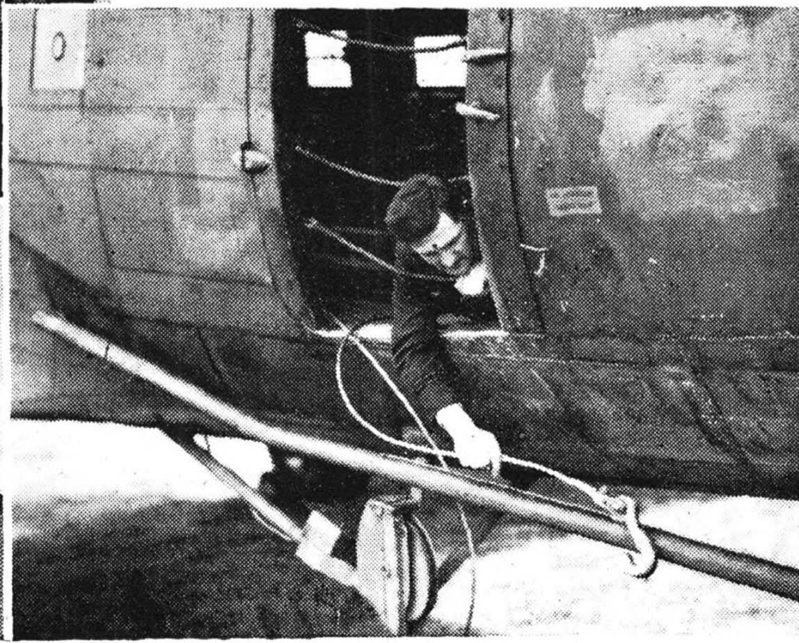
By employing the hysteretic qualities of nylon rope it is possible to make snatch pick-ups of stationary gliders without the tug aircraft landing. This has proved very useful for reclaiming empty gliders after an airborne landing and for clearing casualties from country unsuitable for making airstrips. These training photographs show (top left) attaching the tow-rope to a Hadrian glider; (left) the method of pick-up by Dakota as it flies over; (right) the hook and pick-up apparatus being examined.
