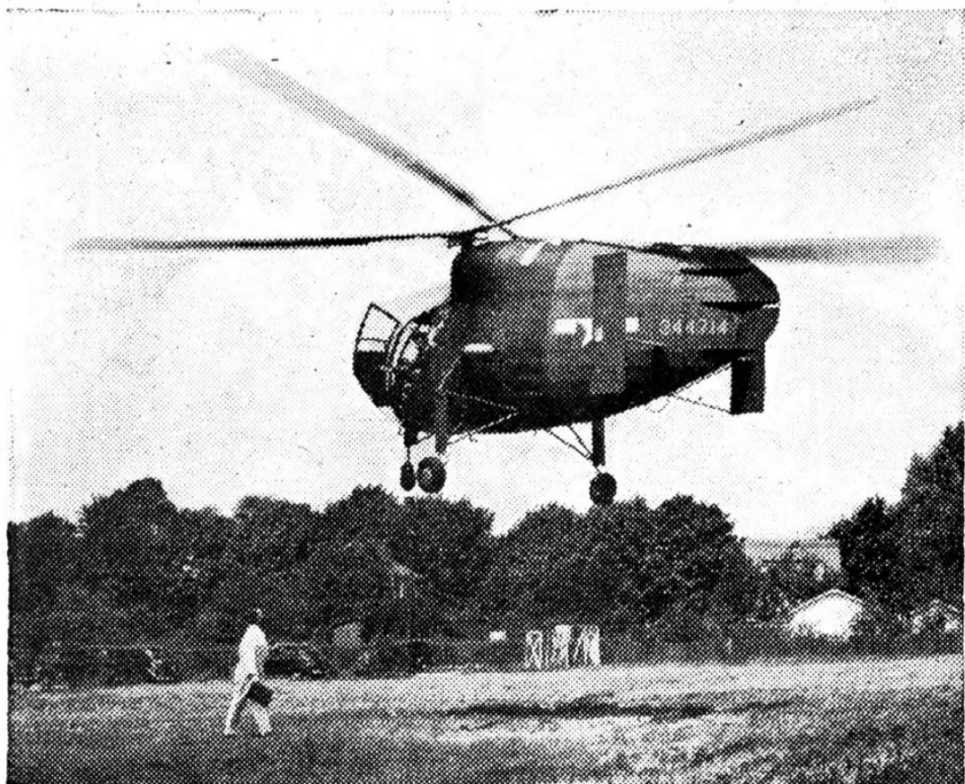
Vertical and horizontal stabilisers occupy the place of the more usual tail rotor.
