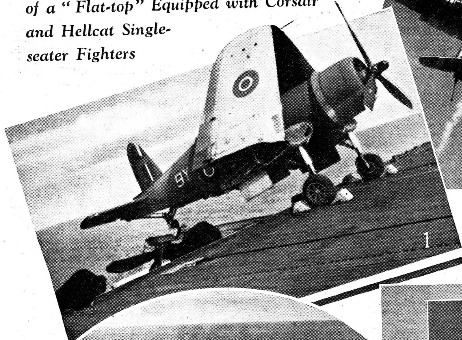
1. To economise in the limited deck space of the escort carrier, the tail wheel of this Corsair is supported on an outrigger projecting beyond the flight-deck. 4. Aircraft damaged beyond repair are dumped into the sea. This badly
