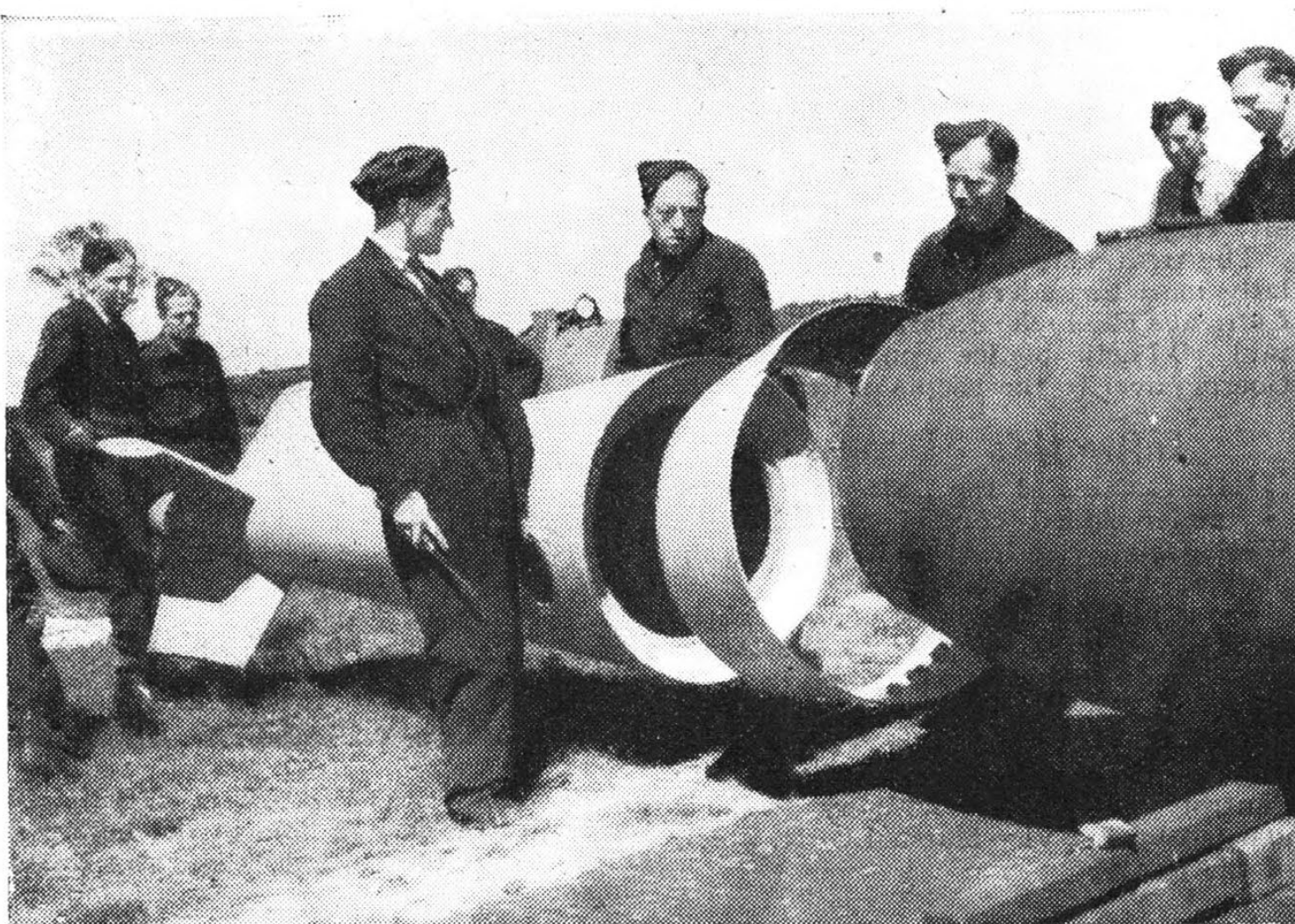
IT NECESSARILY FOLLOWS: Tails with aerofoil fins which set the R.A.F.'s super-heavy bombs spinning ensure even greater accuracy. The method of their attachment is clear from this picture.
