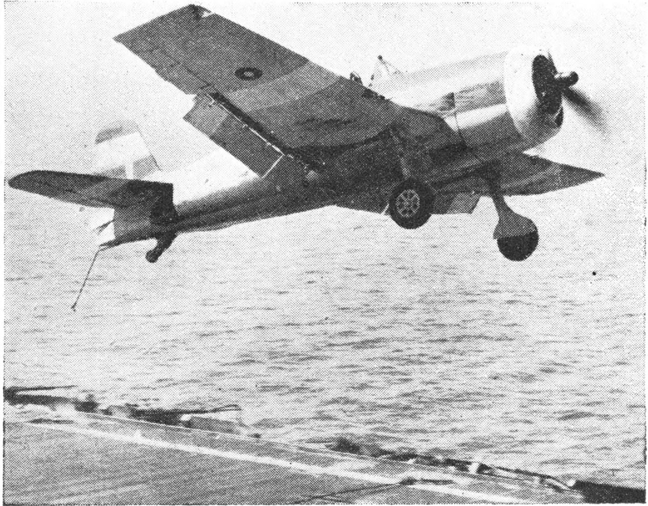
SECOND ROUND: A F.A.A. Hellcat flies round its escort carrier for a fresh approach, with undercarriage, flaps, and arrestor hook down. This Hellcat bears recognition stripes similar to those on the Thunderbolt.
