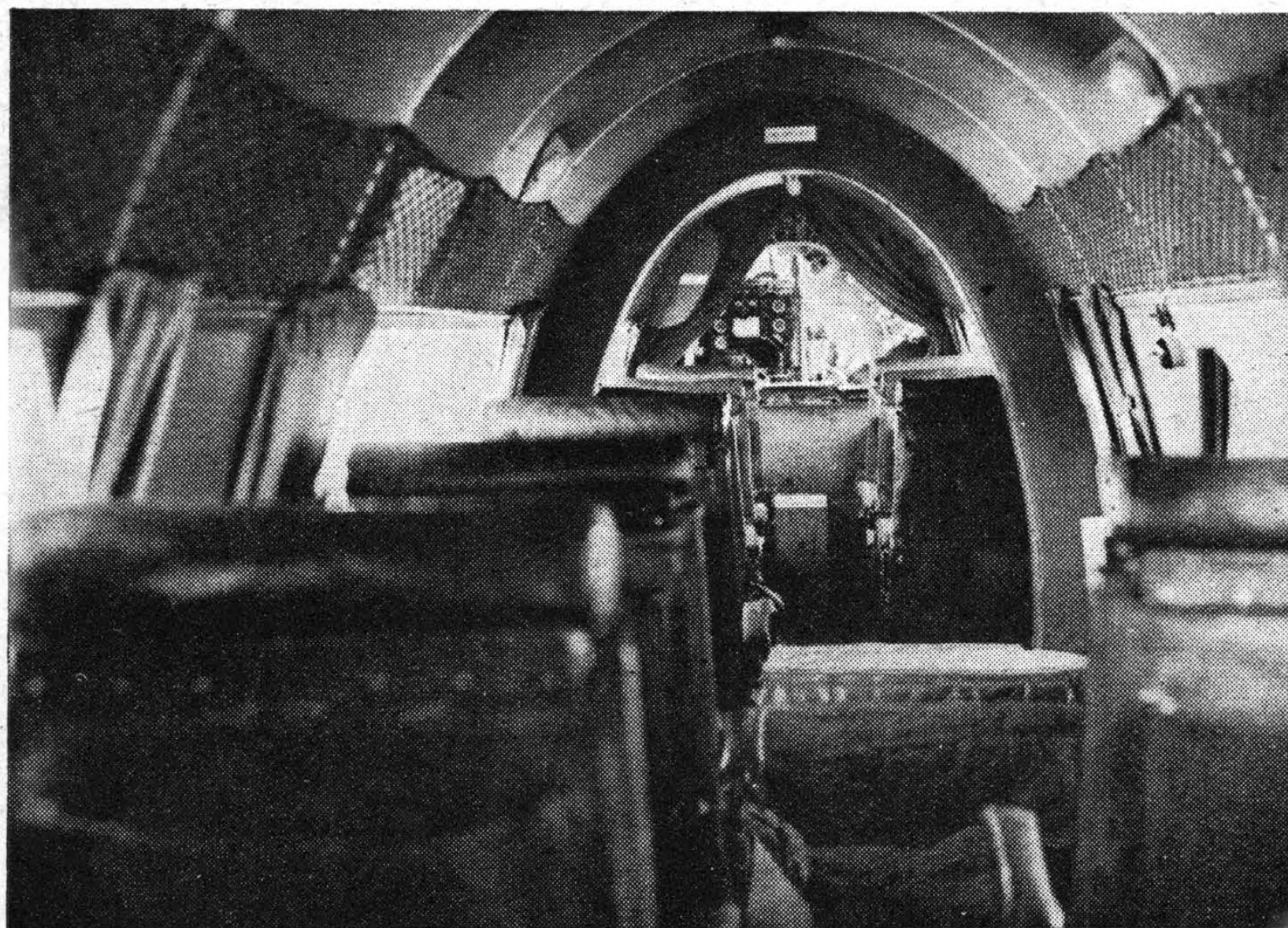
The absence of cross-bracing in the geodetic construction of the fuselage makes the Vickers-Armstrongs Warwick particularly adaptable to a passenger aircraft. It enables a good streamline form to be used in a most efficient manner.
