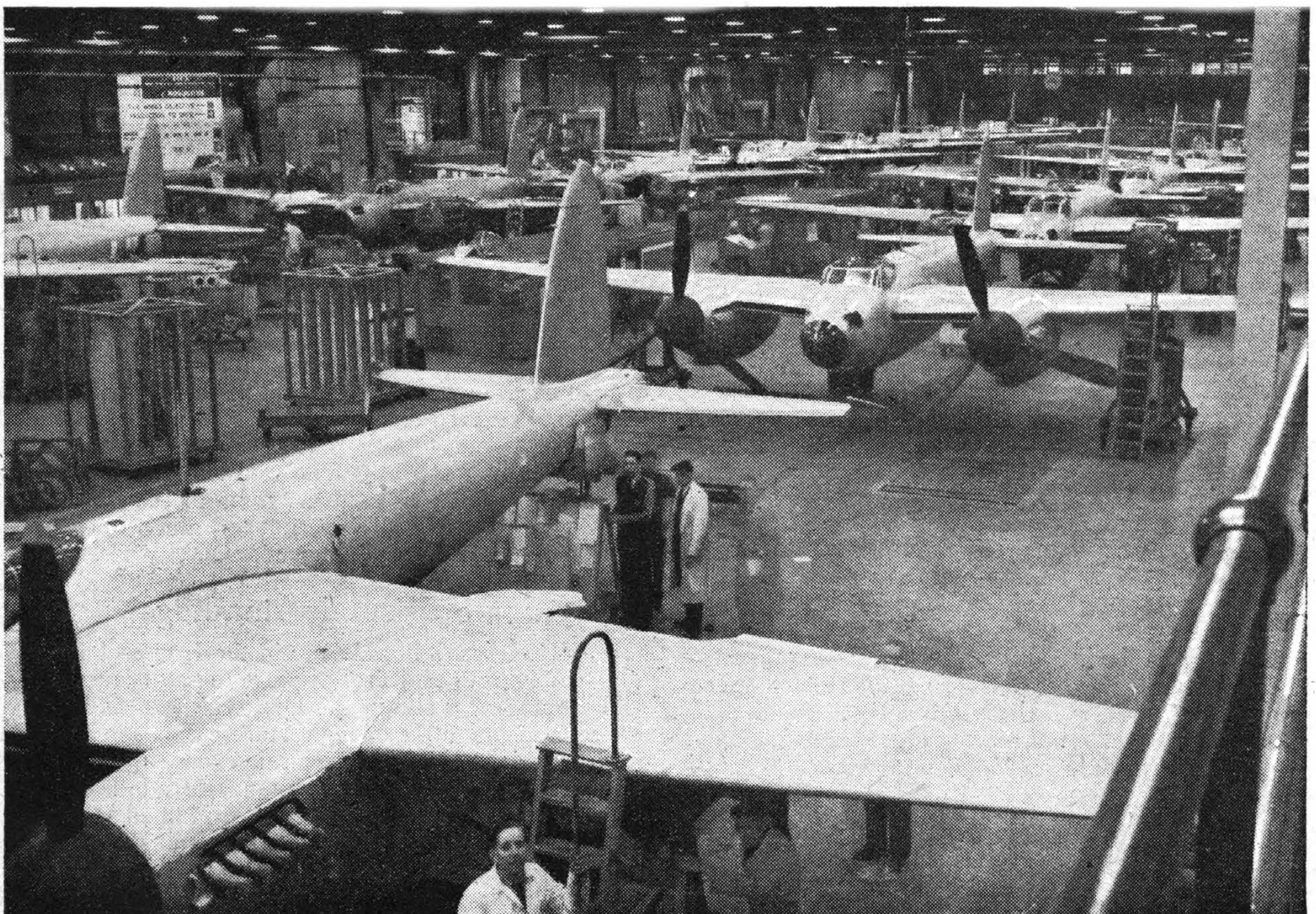
DOMINION EFFORT : A line of Mosquitoes coming through in the final assembly shop of the De Havilland Aircraft Company's Canadian factory.
