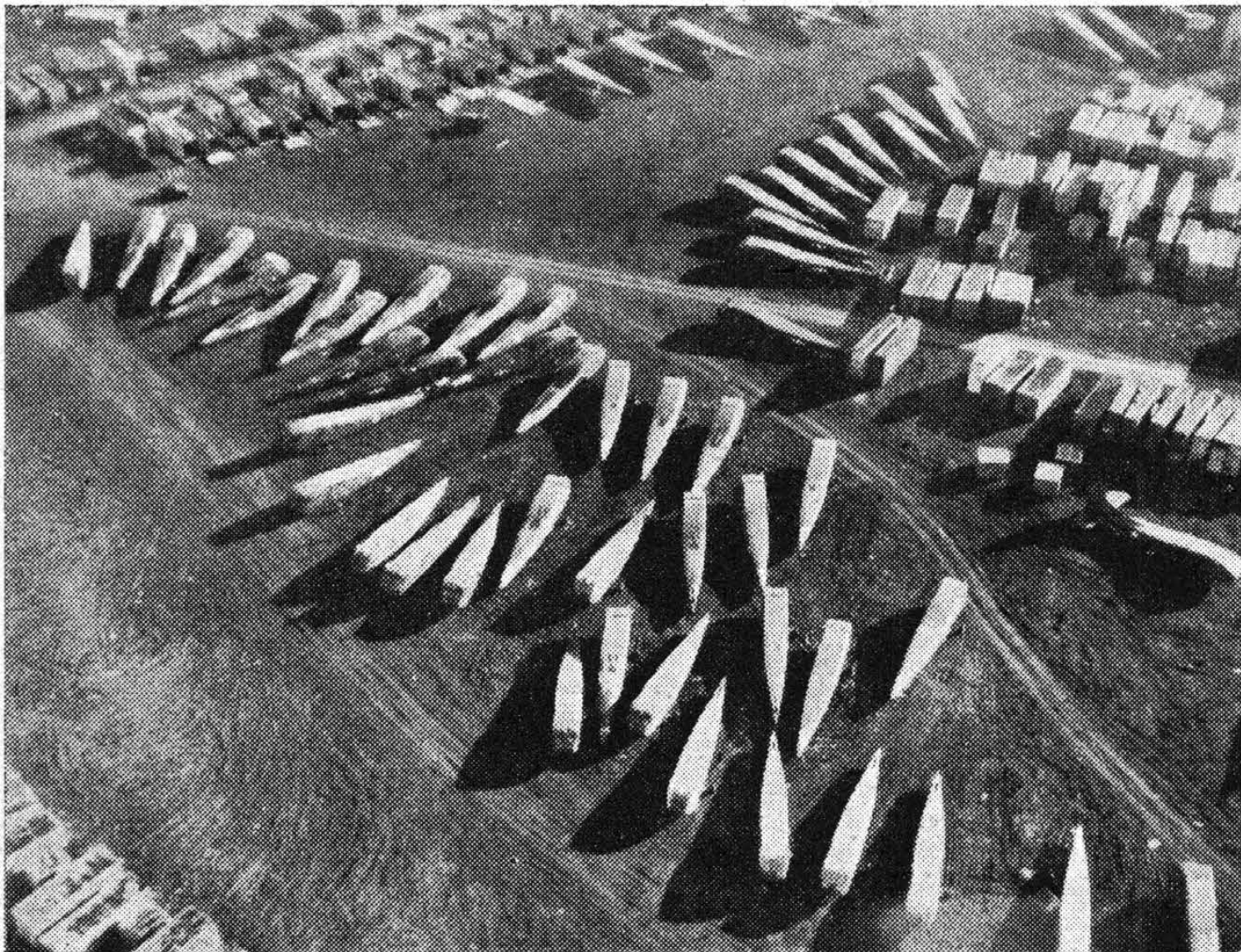
WINGS TO FOLLOW: Looking anything but aeronautical in this "upstairs," view of a corner of a U.S. Ninth Air Force station, the fuselages of CG-4A gliders await their wings.
