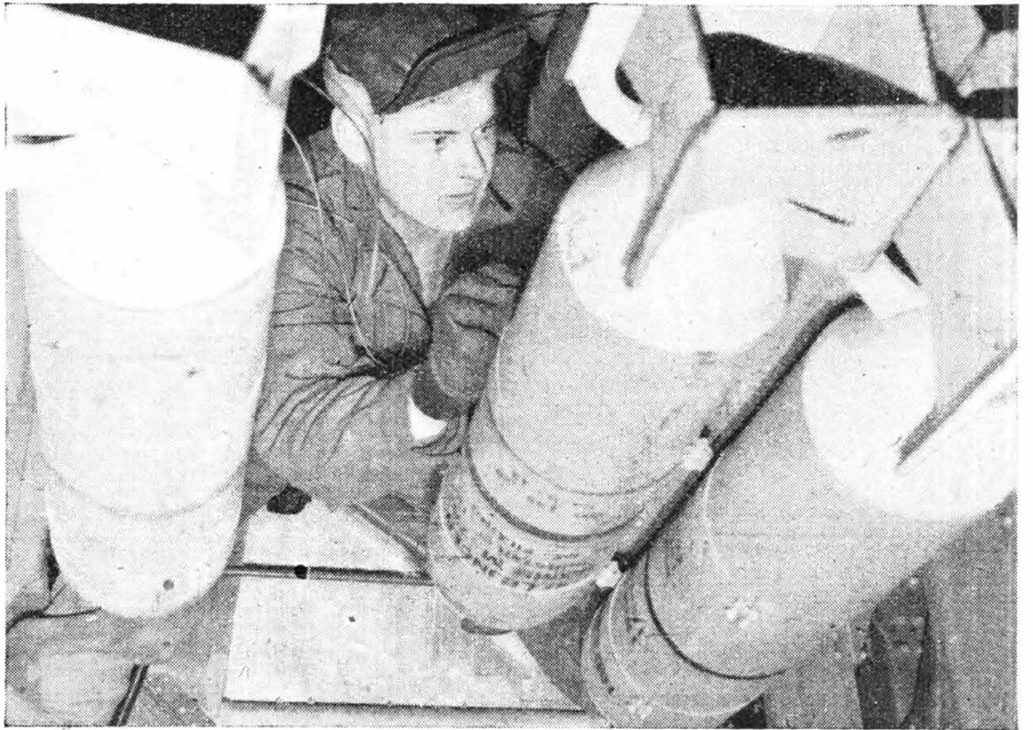
Arming 100 lb. incendiary bombs in the bomb bay of a Flying Fortress.
