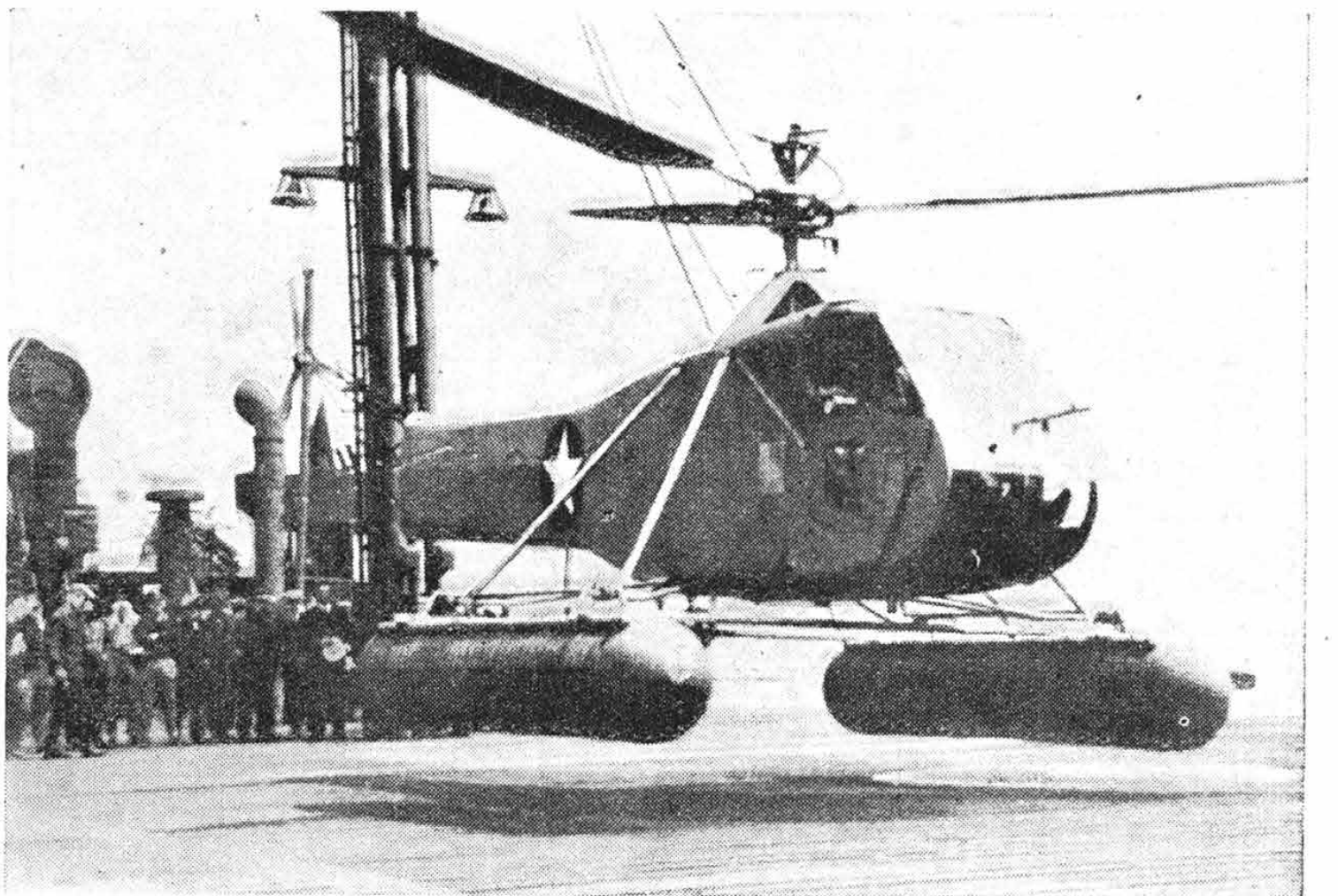
The Sikorsky R4 helicopter, shown here landing on a 20ft.-square deck, is the first helicopter ever to go into production for military purposes.
