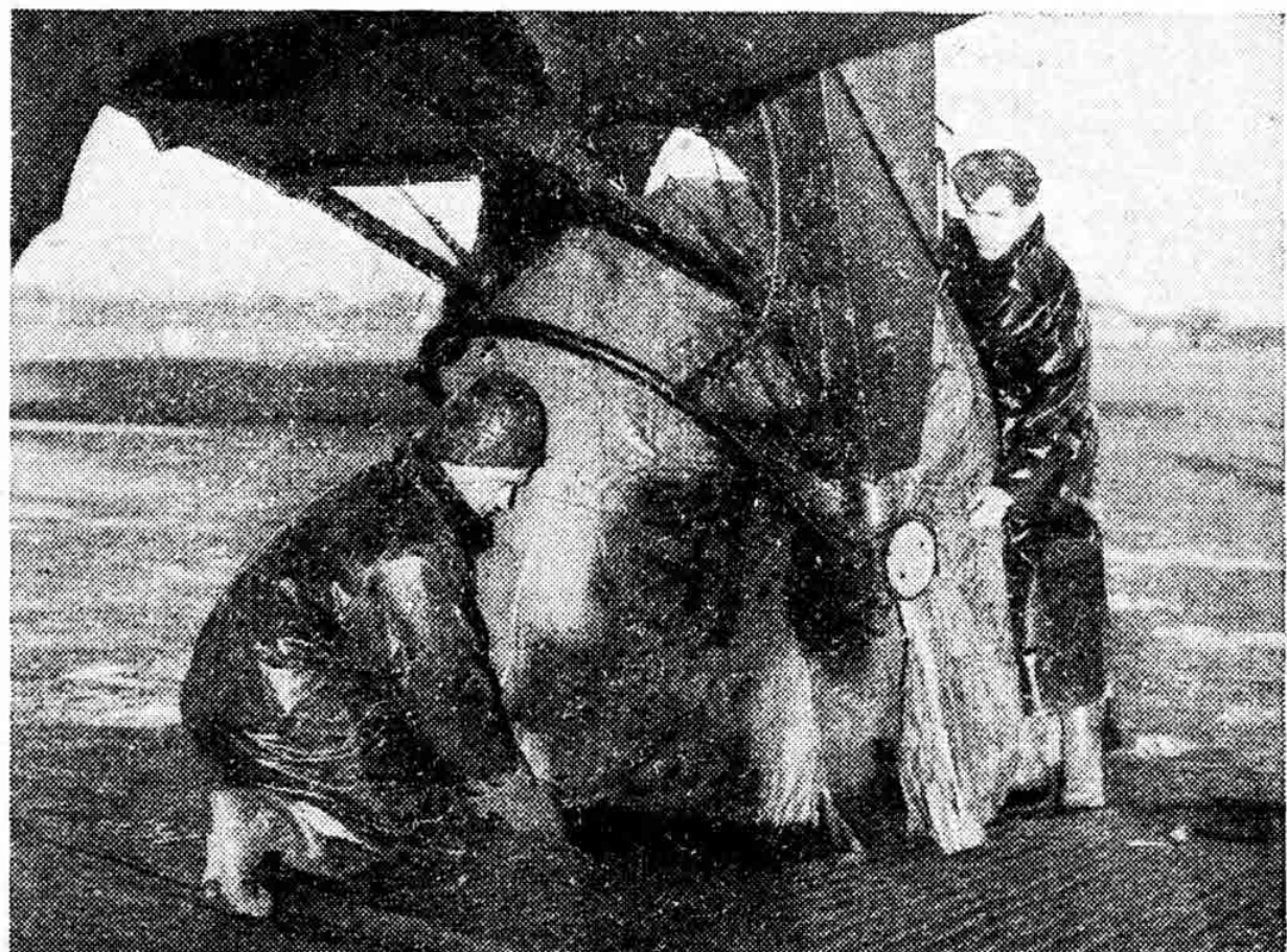
BOOTES FOR THE HALIFAX. —Two members of the ground crew place protective oilskin covers over the wheel of a Halifax. The photograph shows clearly the details of the sturdy Messier undercarriage.
