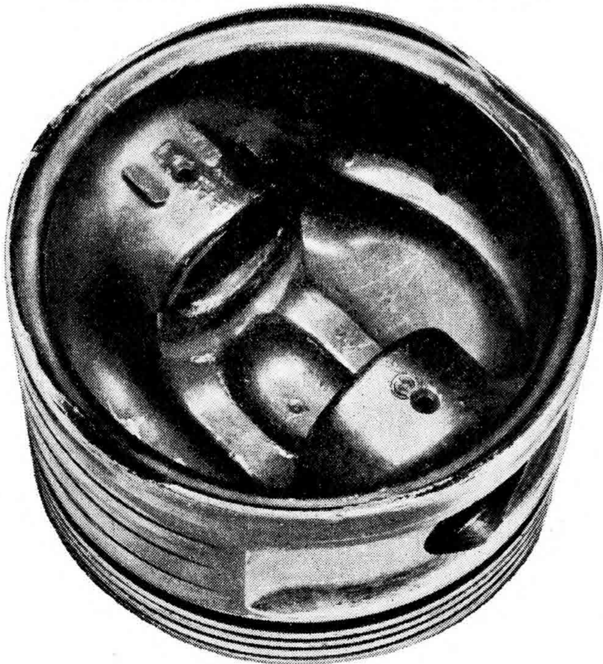
Piston from Bramo-Fafnir 323 P1 radial motor.
