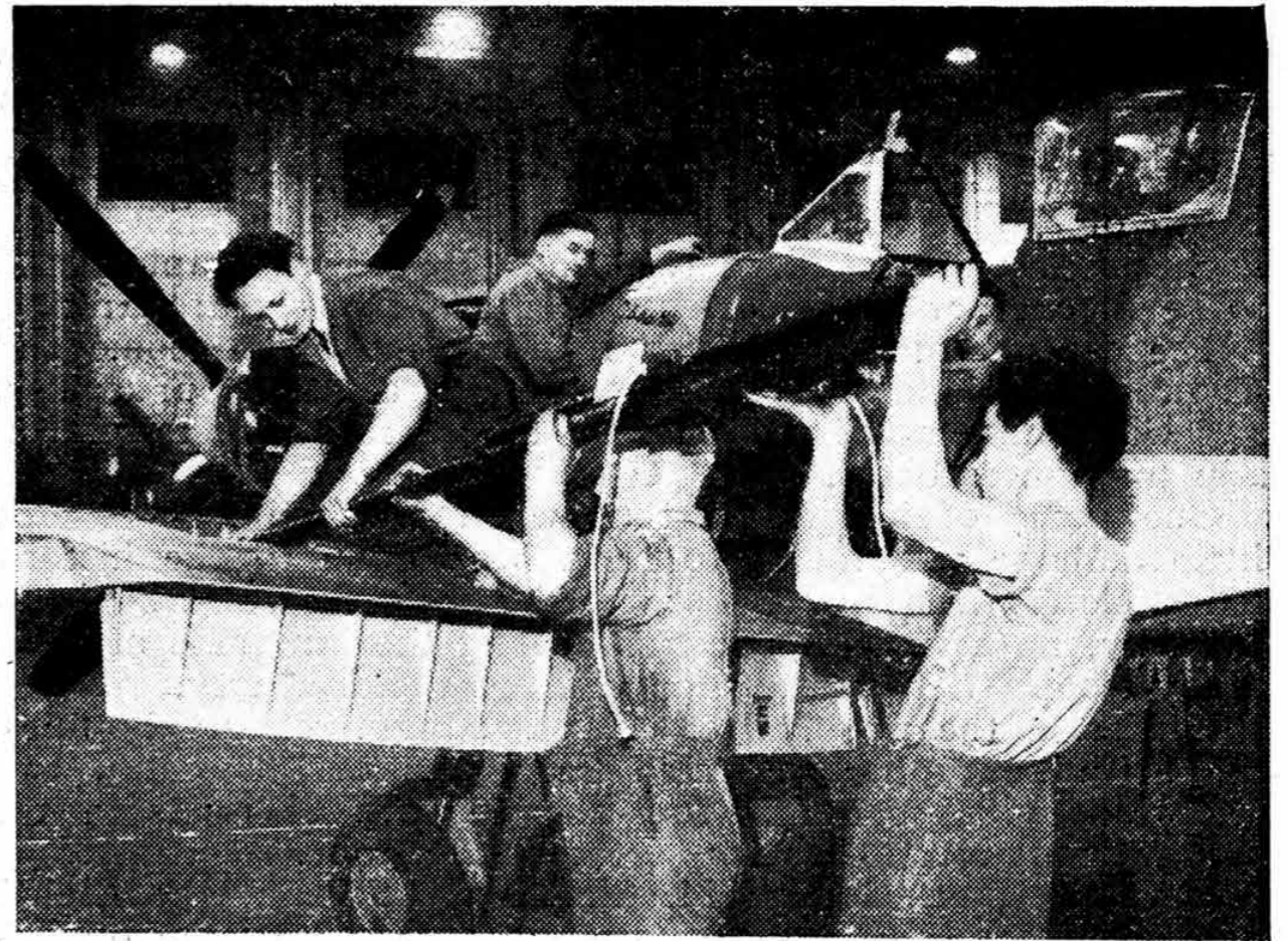
GIVING IT THE WORKS. —Workers at a British aircraft factory fitting a 20 mm. British Hispano cannon in the wing of a Spitfire IX. This photograph also shows the split flap clearly.
