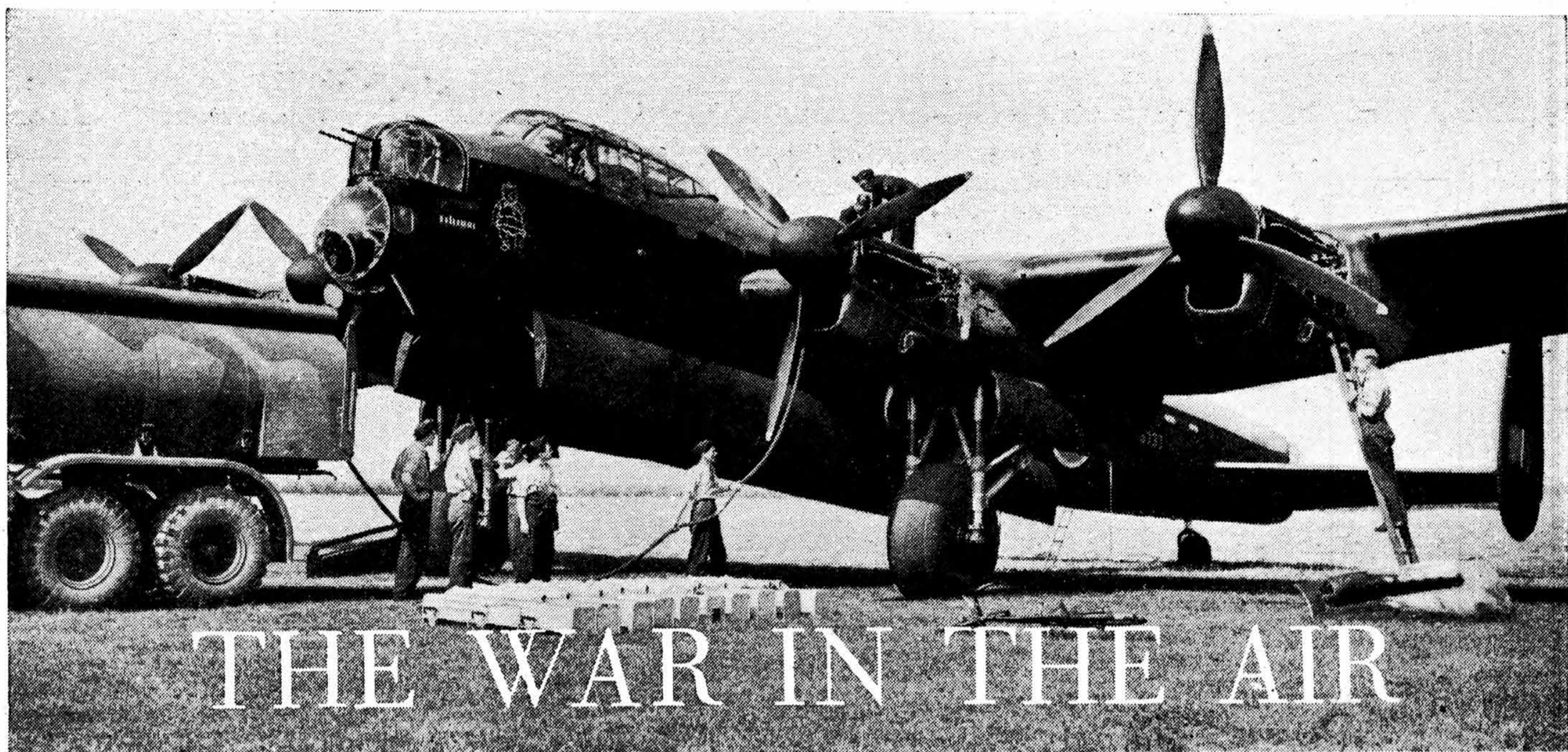
QUENCHING THE MONSTER'S THIRST. —An Avro Lancaster I being refuelled by a petrol bowser while the Rolls-Royce Merlin motors are checked over by the mechanics. Lancasters are being used on all Bomber Command's night attacks on Germany.
