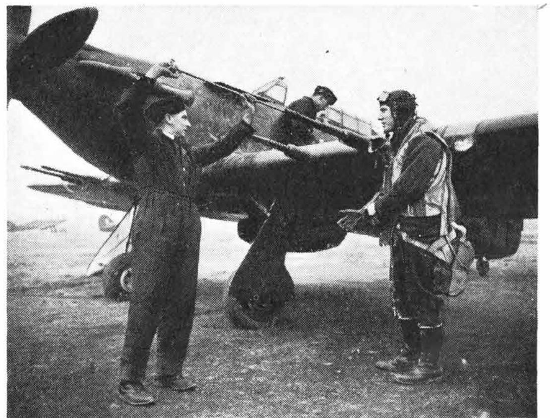
THE ARMOURER'S PIPE CLEANER. —Last minute pull through of the Hispano cannons of a Hurricane IIc night fighter.
