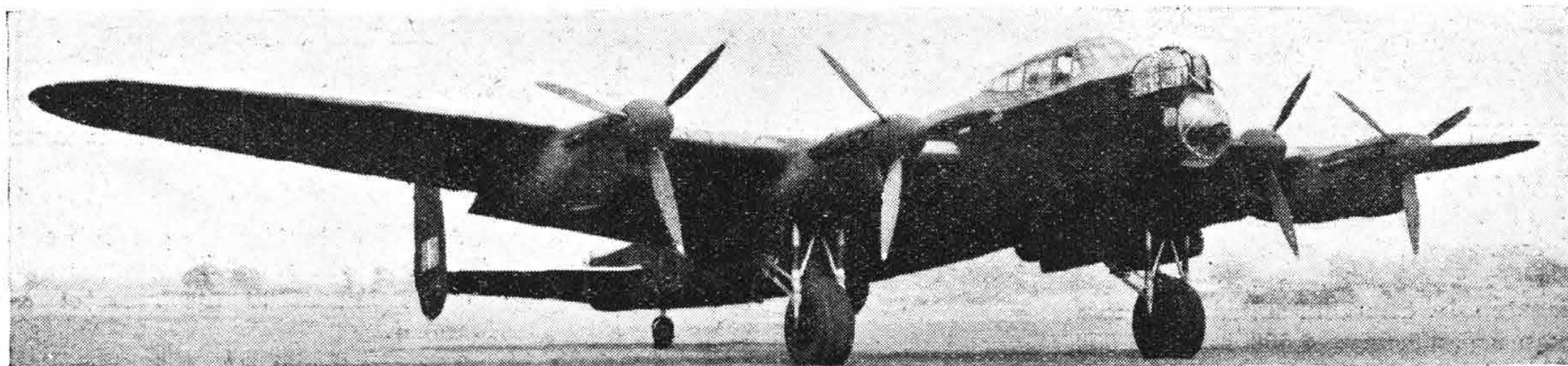
A SMASH HITTER. —The great Avro Lancaster, which has taken part in many large-scale raids on German centres of production. The Lancaster is to be distinguished from the Halifax by rounded wing-tips, taller fins and rudders, and smoother lines generally.
