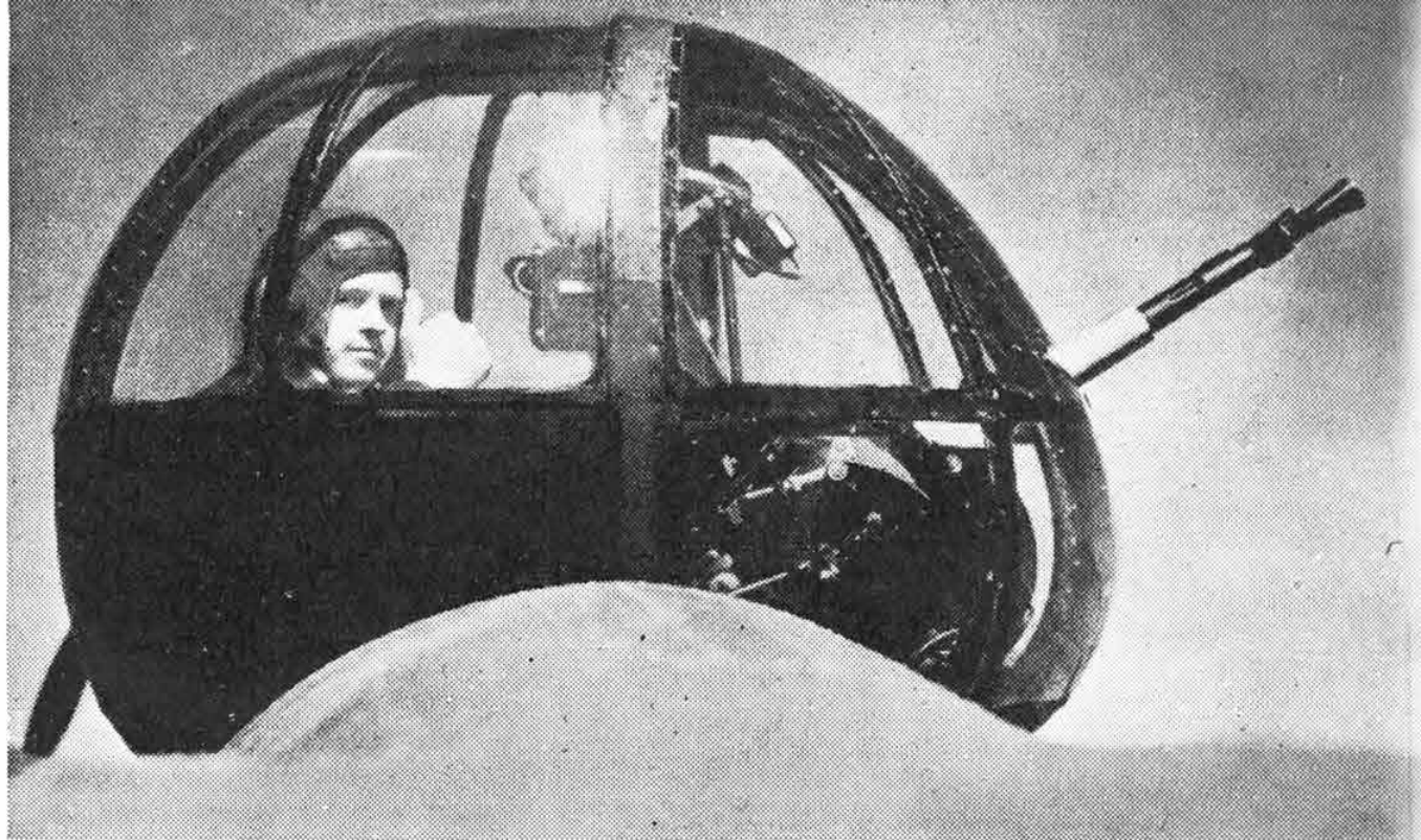
BUBBLE TURRET. —The electro-hydraulically operated gun turret made by Boulton Paul Aircraft Ltd. which has been fitted to many aeroplanes and is here seen on an American Lockheed Hudson, in service with Coastal Command. This type of turret is used also on top of the Halifax II.
