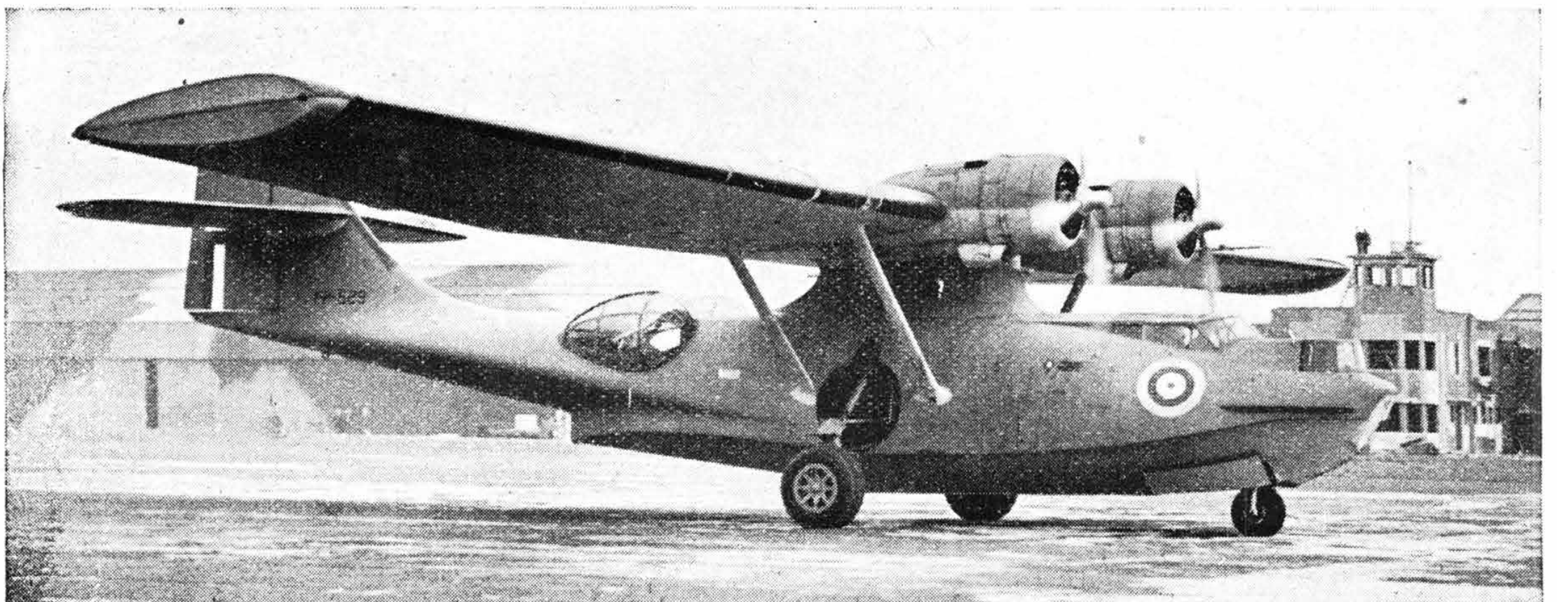
CATALINA AMPHIBIAN. —Consolidated 28-5A tricycle amphibian flying-boats are now in service with the R.A.F. and are reported from Canada to have been named the Cansos. The tricycle undercarriage makes the Cansos equally easy to operate from land or sea stations. It is in service in the U.S. Army under the designation OA-10.
