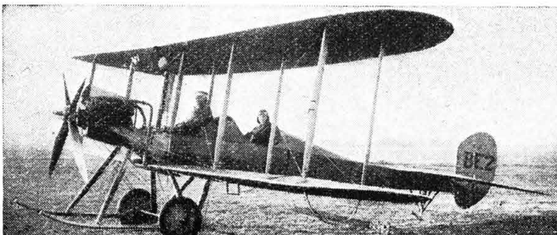
DE HAVILLAND FAMILY.—(Left) The original B.E.2, (70 h.p. Renault motor) of the Royal Aircraft Factory, which was designed by Geoffrey de Havilland, who is seen sitting in the pilot's seat at the back. (Right) The D.H. 82A (130 h.p. D.H. Gipsy Major motor), the Tiger Moth. The B.E.2, as an officially designed aeroplane was not entered in the Government's Military Trials of 1912, but flying hors-de-concours proved itself the best type of that year. The prototype was produced in January, 1912, and had about the same performance as the first de Havilland Moth.
