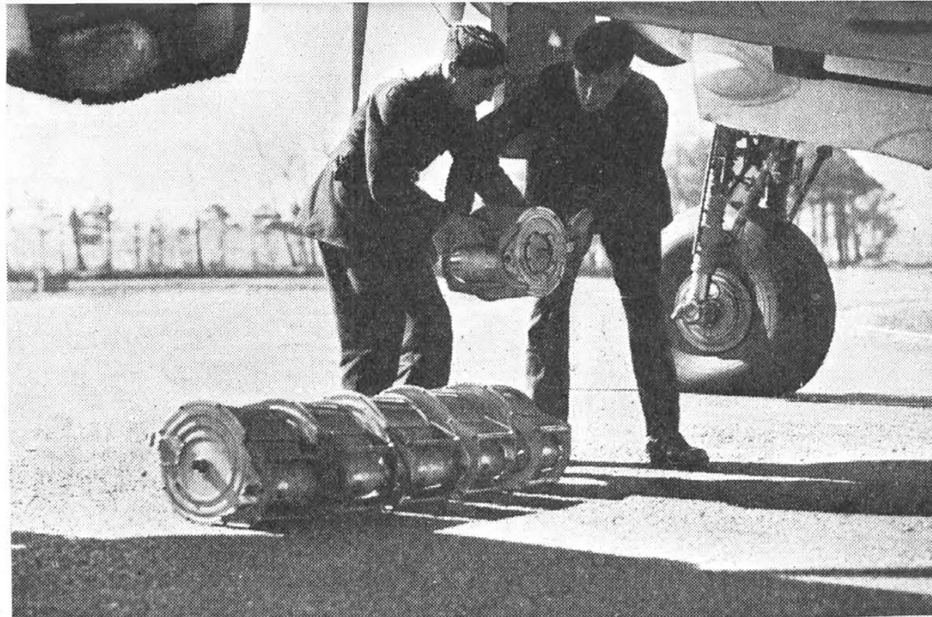
CANISTERS OF CANNON FODDER.—Loading up a Bristol Beaufighter with drums of ammunition for its four 20 mm. shell guns.
