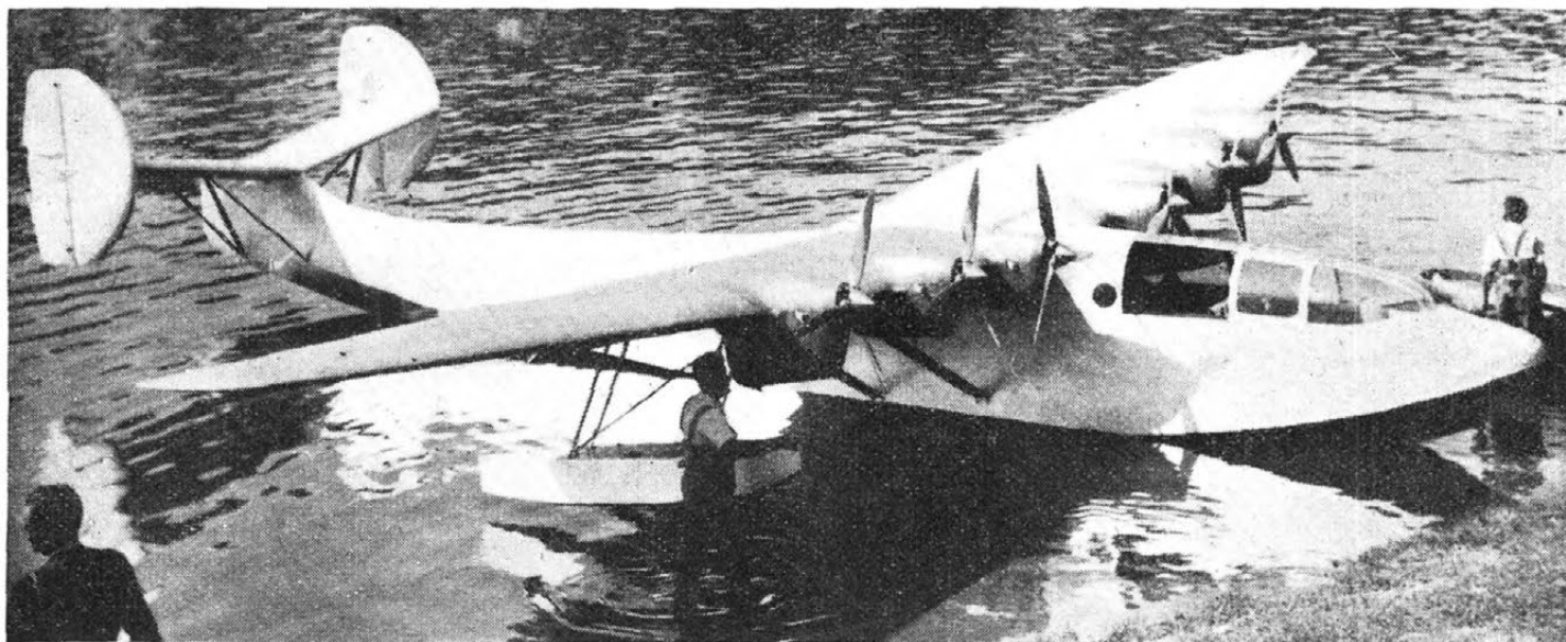
THE PROTOTYPE.—The Potez 160, the flying scale model of the new Potez 161 trans-Atlantic flying-boat which has recently been completed in France. According to reports from Vichy the Potez 161 is powered with six 1,000 h.p. Hispano-Suiza motors, has a top speed of 225 m.p.h., a cruising speed of 188 m.p.h. and a range of about 5,200 miles. It was built at Sartrouville, near Paris, and is to be flown to Biscarosse for its trial flights. The model, the 160, was powered with six 40 h.p. Train motors and was shown at the Paris Aero Show in 1938.
