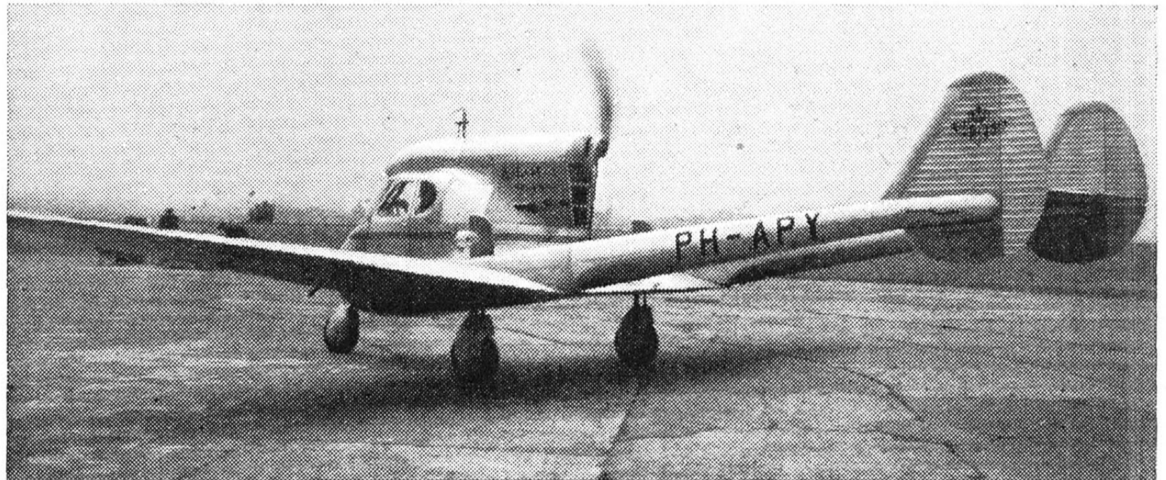
The unorthodox Stearman-Hammond Y which K.L.M. used before the war to train their pilots in the art of tricycle landings. It is a two-seater with a 150 h.p. Menasco engine and numerous interesting features.
