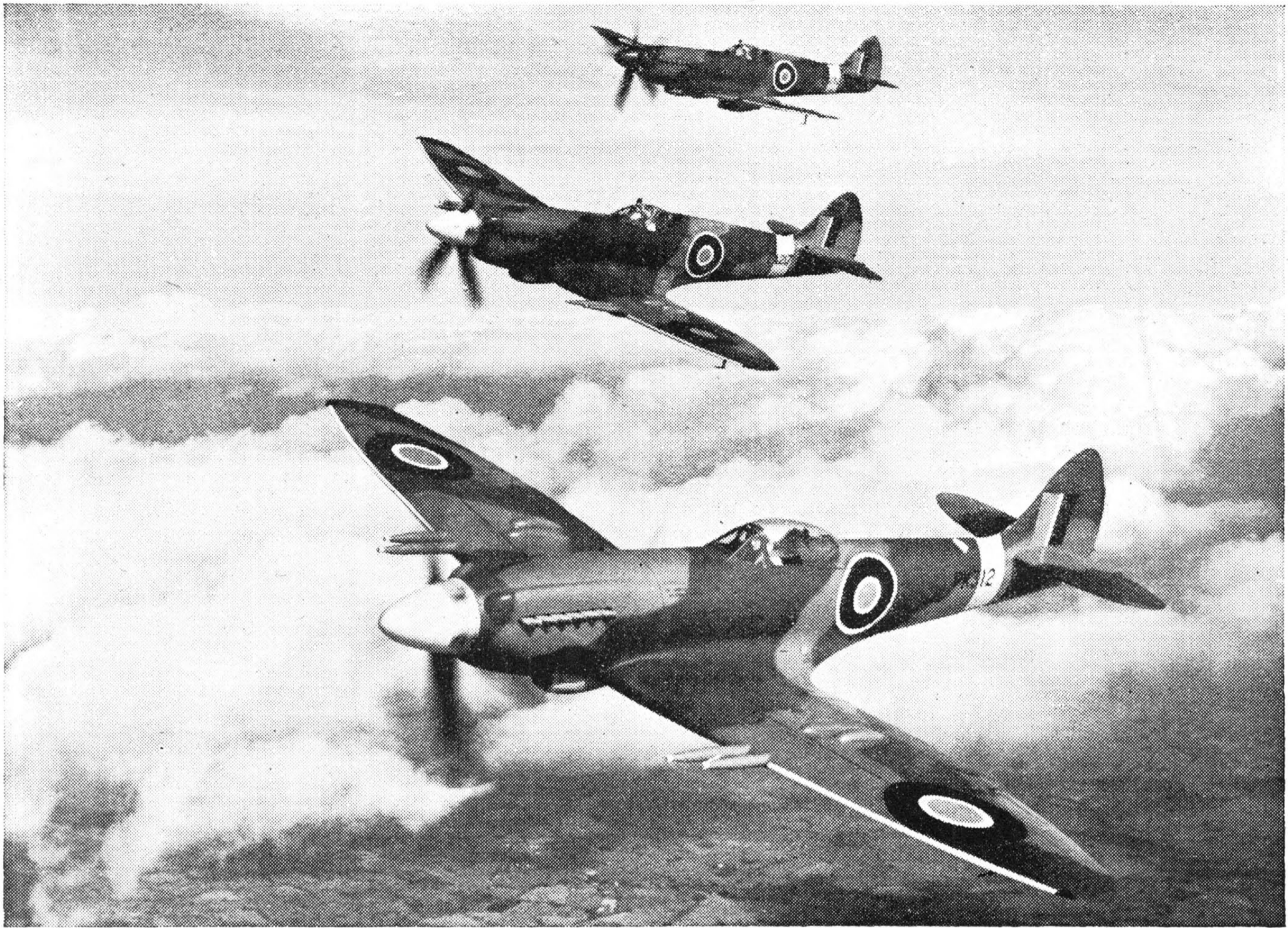
THE LAST WORD in Spitfire design is embodied in the Mark XXI and XXII, making up this formation. Only visible difference in these Griffon-engined types is the Mark XXII's bubble canopy (nearest the camera).
