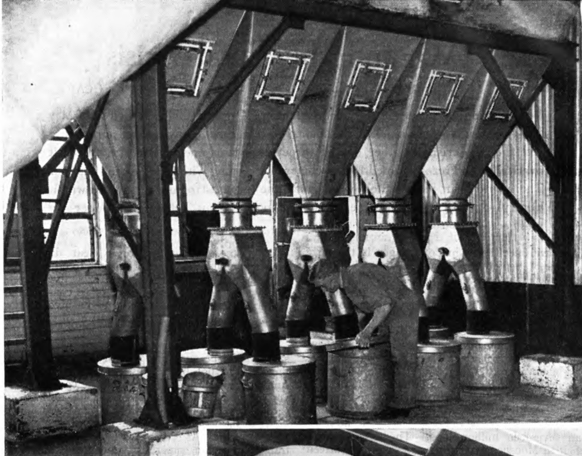
The spray-drier to which the extract is pumped after filtration.
