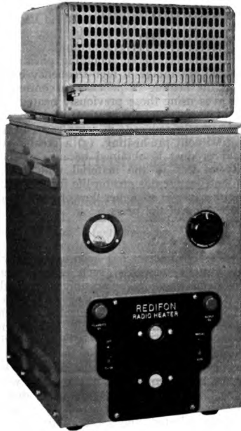
Fig. 2. —Small high-frequency heater for general production with cage for pellet heating.
