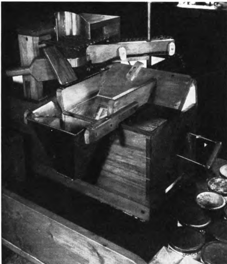
The fluorometer with the receiver cup in position for the preliminary moisture determination.
