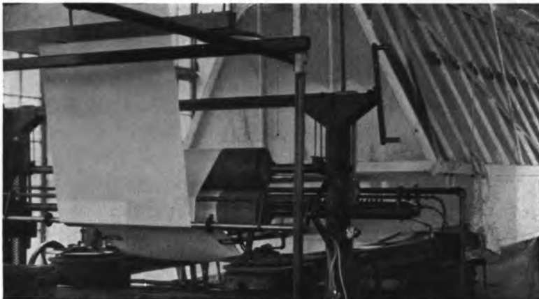
Fig. 1. One of the early types of preshrinking machines developed by Sanford L. Cluett
