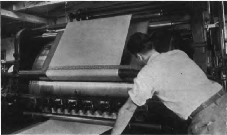
Fig. 2. View of modified Palmer employed in compressive shrinkage process
