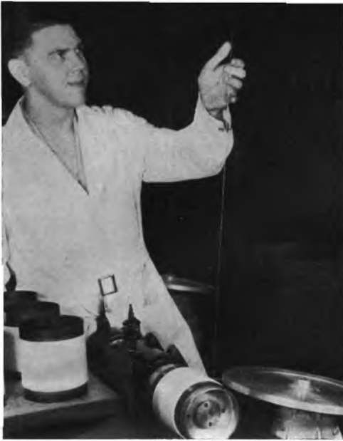
The continuous filaments pass over a rotating disk and are wound on spools
