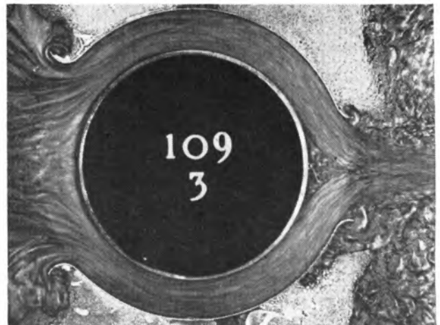
FIG. 9 VISUAL-FLOW PATTERN, REYNOLDS NUMBER OF 3550
