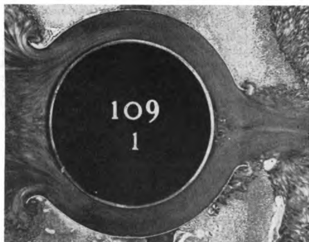
FIG. 10 VISUAL-FLOW PATTERN, REYNOLDS NUMBER OF 13,820
