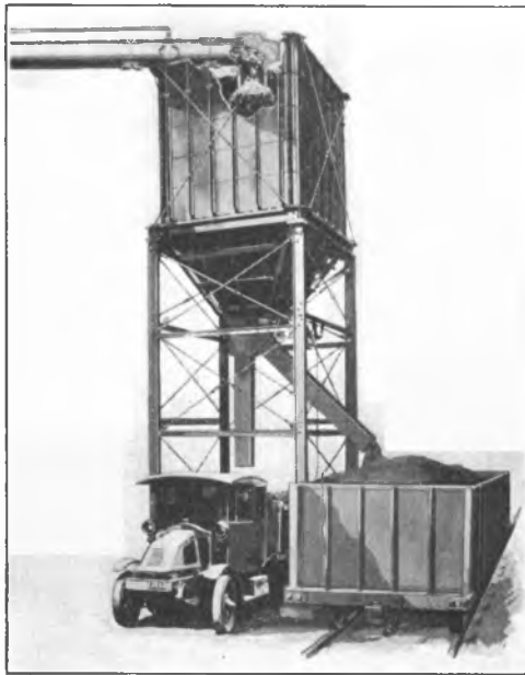
FIG. 29 CAST-IRON-PLATE ASH BUNKER
