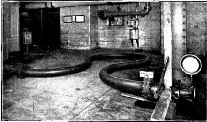
FIG. 15 SET-UP FOR TEST OF ELASTICITY OF 6-IN. DOUBLE-OFFSET EXPANSION U-BEND
