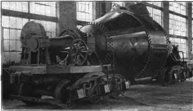
FIG. 4 PUGH MIXER-TYPE HOT-METAL CAR
