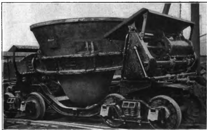
FIG. 5 SLAG CAR AND LADLE
