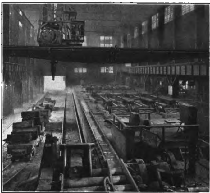
FIG. 10 GENERAL VIEW OF SOAKING PITS, INGOT TILTER AND TONG CRANE
