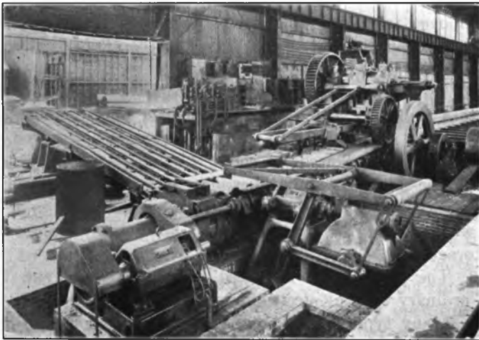
FIG. 12 BILLET CONVEYOR AND GRASSHOPPER PUSHER
