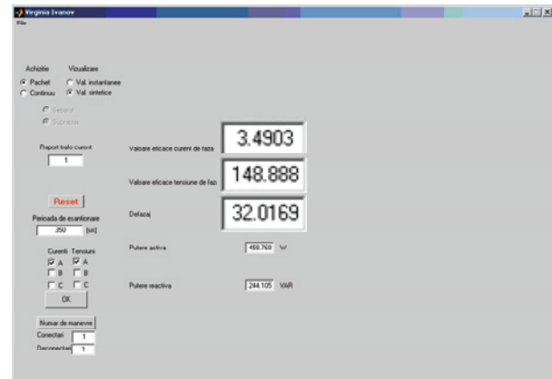
Fig.6. Synthetic values for the phase A of an inductive load with micro-system
