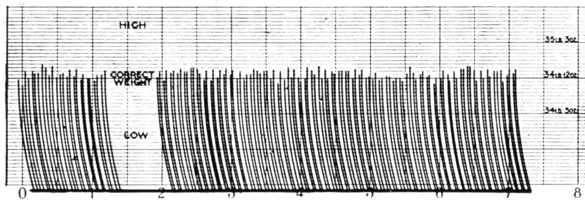
Electrically Recorded Graph of an actual Lap Test under mill conditions
