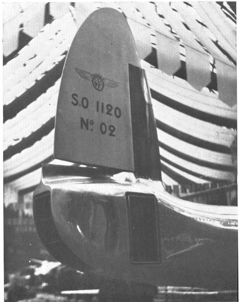
Fig. 24. —The use of exhaust gas coupled with deflectors and with the rudder was used in the first Cierva helicopter. In the SO-1120 the extra volume of the turbine exhaust and the almost complete absence of torque make it a practical control system
