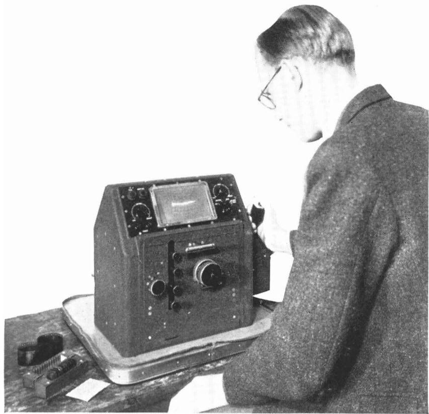
Fig. 6.—Assessing a V-g recorder slide in the assessor designed and built at the Royal Aircraft Establishment. The image of the small slide is magnified and projected on to the screen for the operator to read, after which he will photograph it for record purposes by simply pressing the camera press-button switch in his right hand. A batch of slides in transit case is on the table to the left
