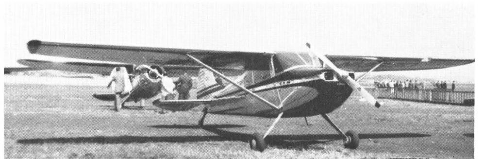
Fig. 5.—A type that is lacking in Great Britain, the four-seater luxury aircraft of good performance. The Cessna 170 for 1951 is a very clean little aeroplane in which the pilot's view is considerably better than on some of the company's earlier models
