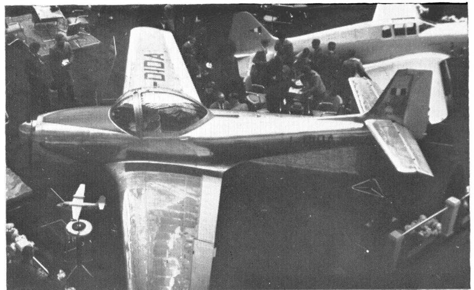
Fig. 18.—The Piaggio P-148 is probably the best-looking three-seater trainer yet built. By using a long rear fuselage the designer seems to have overcome the awkward spinning characteristics common in such layouts, where the large cockpit canopy interferes with the air flow
