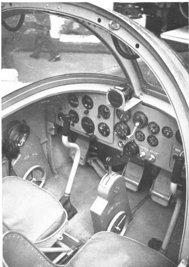
Fig. 19.—The cockpit frame of the P-148 is sturdy and forms a crash arch, but does not interfere with the view. Flying controls, throttle, mixture and trim are duplicated, but instruments are not. The handle in the middle of the dash is the manual pitch control for the Piaggio propeller
