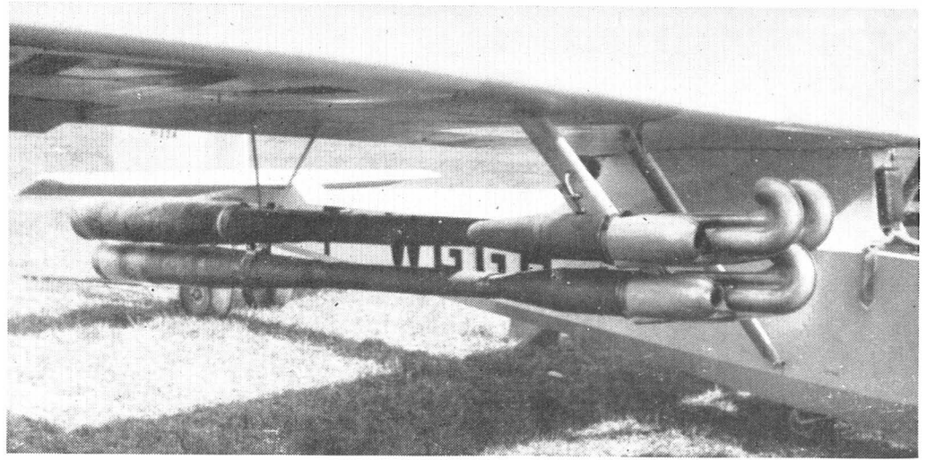
Fig. 31.—The SNECMA Escopette (Blunderbuss) in a triple unit under the wing of an Emouchet glider. The front mounting strut carries the fuel pipes and ignition leads, while the rear mounting is little more than a 'steady'. Discolouration of the main body and the recuperators shows where the parts run hot
