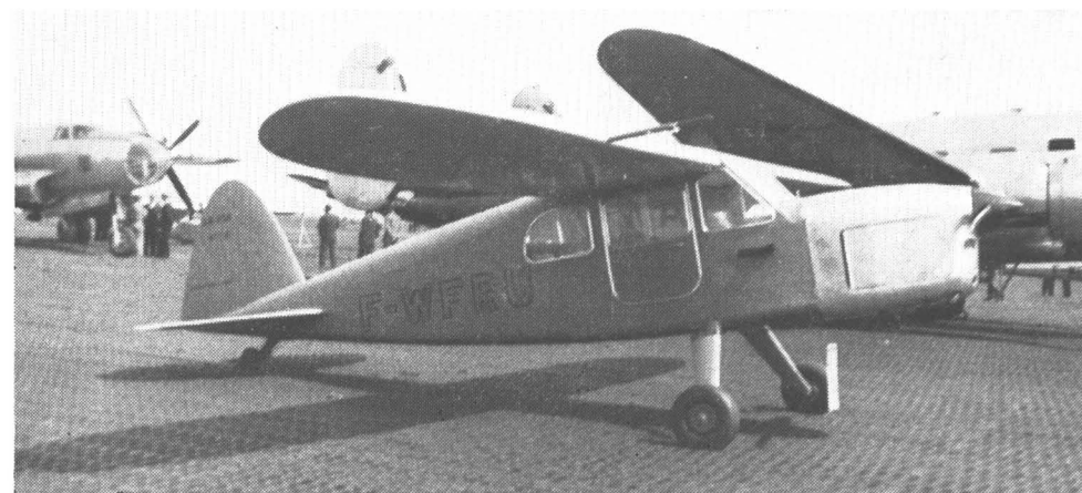
Fig. 1.—The Paul Aubert Cigale Major is a new version of a pre-war light aeroplane. Its clean lines and neat engine cowling (which opens backward in two large panels, with two small inset upward opening doors for priming, etc.) show well in this view
