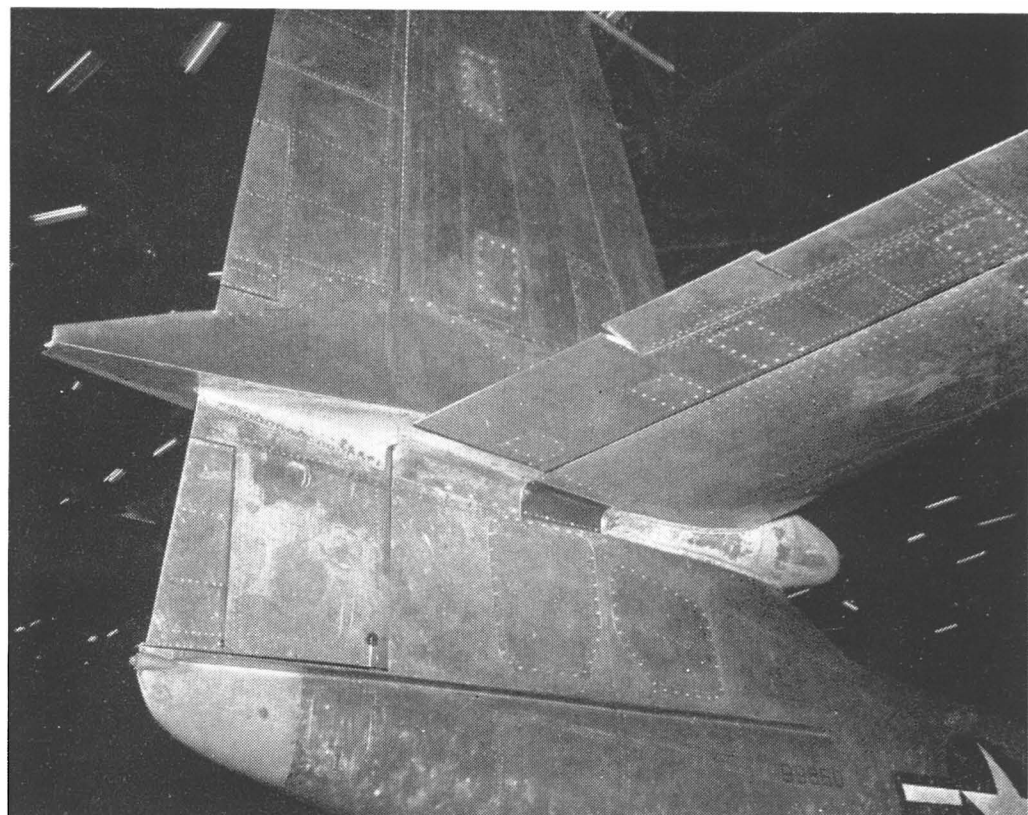
Fig. 6.—The addition of a very large fillet to the bullet fairing
