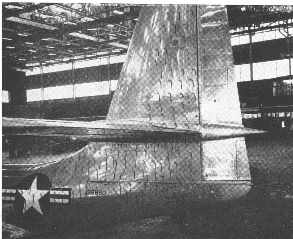
Fig. 5.—A tail fairing added to the bullet
