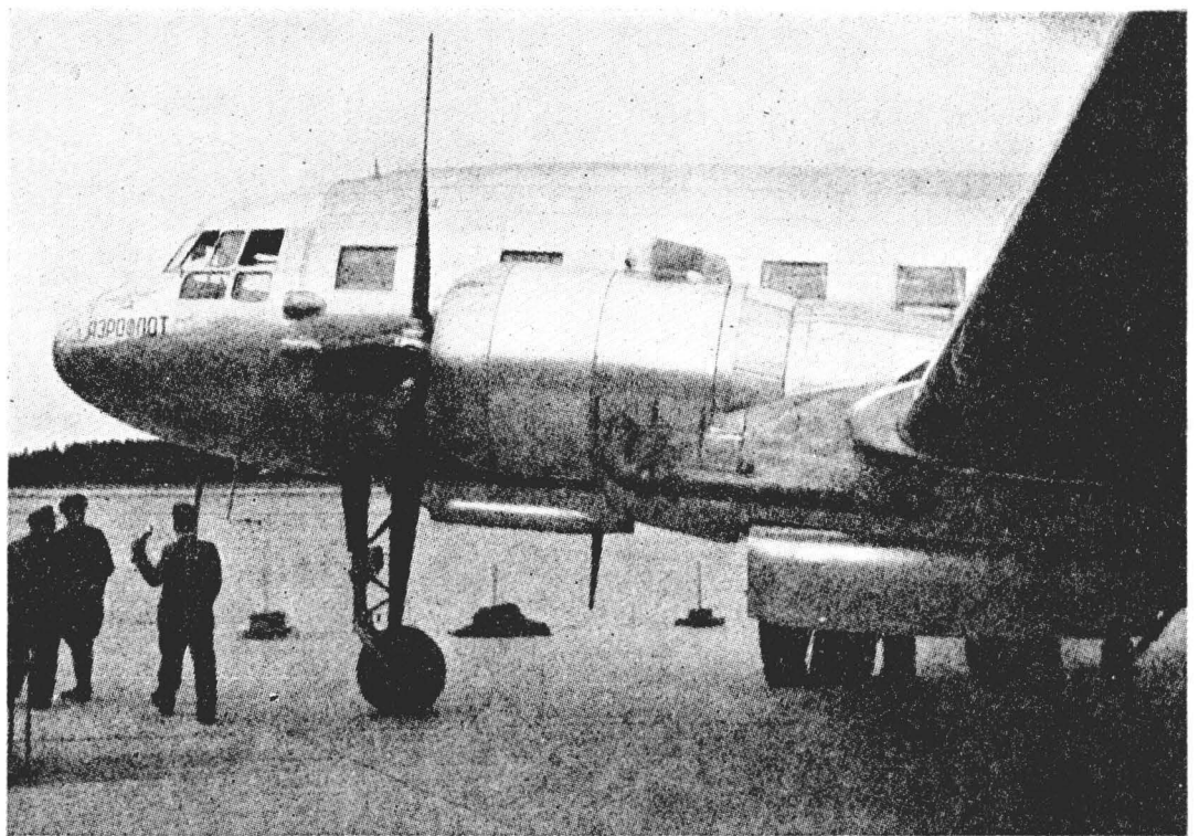
Fig. 7.—New photographs of the standard II-12 medium range air liner and troop transport, which has a crew of 5 and 27 to 32 passengers. The engines are ASH-82 fourteen cylinder two-row radials with two-speed superchargers giving 1,700 h.p. Span 31.7 m. (104 ft.); length 21.3 m. (70 ft.); height 6.25 m. (20 ft. 6 in.); gross weight 17,250 kg. (38,000 lb.); pay load 3,000 kg. (6,600 lb.) max.; max. speed 407 km.p.h. (253 m.p.h.) at 2,600 m. (8,530 ft.); cruising speeds 320 km.p.h. (200 m.p.h.) at sea level, 350 km.p.h. (217 m.p.h.) at 2,600 m (8,350 ft.); range 1,250 km—4,000 km. (775 miles—2,480 miles). A freighter version is said to have been built with a maximum load capacity of 4,000 kg. (8,820 lb.)
