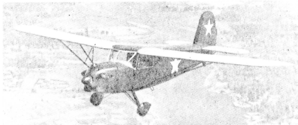
Fig. 15 (below).—Built in 1945, the Yak-14 is a little known communications monoplane in service both as a land, sea and ski plane. 145 h.p. M-11 engine in a helmet cowling. Span 12 m. (39 ft. 6 in.); length 8.45 m. (27 ft. 8 in.); wing area 22 sq. m. (237 sq. ft.); tare weight 770 kg. (1,700 lb.); gross weight 1,200 kg. (2,650 lb.); max. speed 200 km.p.h. (124 m.p.h.); cruising speed 160 km.p.h. (100 m.p.h.); landing speed 70 km.p.h. (43 m.p.h.); initial rate of climb 3.3 m. sec. (650 ft. min.); ceiling 4,000 m. (13,120 ft.); range 1,000 km. (620 miles)
