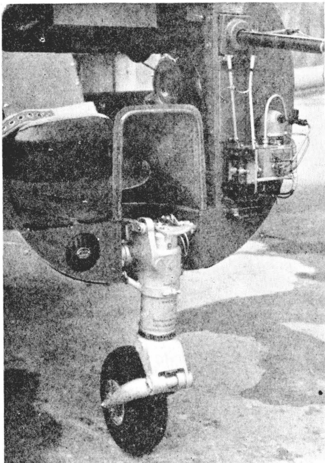
Fig. 17.—The front bulkhead of the fuselage, showing the electro-hydraulic pump unit, Dowty nose-wheel leg and mounting and the end of the control column
