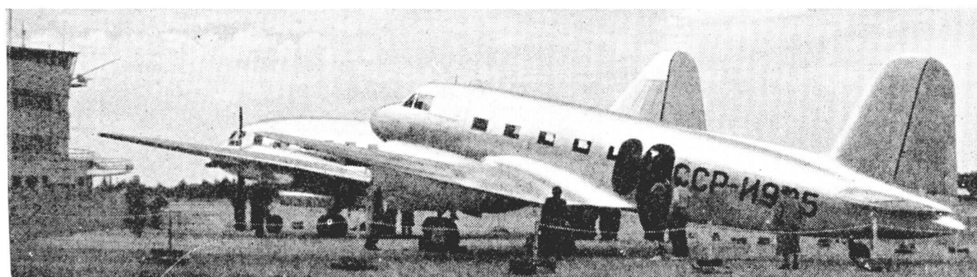
Fig. 16.—Although the Yak-16 all metal feeder liner was exhibited this year at the Polish Air Show, information about it is still conflicting. Inspection of photographs shows it to be of conventional construction and apparently good workmanship—but the exteriors of Russian aircraft are generally better finished than the unseen parts. Statements on accommodation vary and it is not clear whether a total capacity of fourteen is available or that there are ten passenger seats with a crew of two or four. The engines are the ASH-21, a nine-cylinder air-cooled radial, giving 760 h.p. for take-off and rated at 630 h.p.; with two-bladed Visch c.p. propellers. Data, which we give with reserve, are as follows: span 17 m. (56 ft.); length 11 m. (36 ft.); height 3.6 m. (12 ft.); max. speed 310 km.p.h. (190 m.p.h.); cruising speed at 1,700 m. (5,600 ft.) 290 km.p.h. (177 m.p.h.); landing speed 90 km.p.h. (50 m.p.h.); service ceiling 5,000 m. (16,400 ft.); range 1,000 km. (620 miles)
