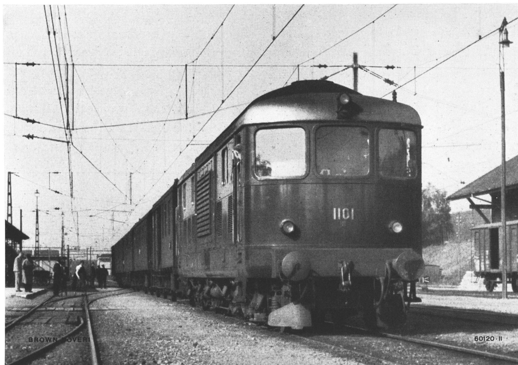
Fig. 151. — The gas-turbine locomotive at a station on the line it is serving.
