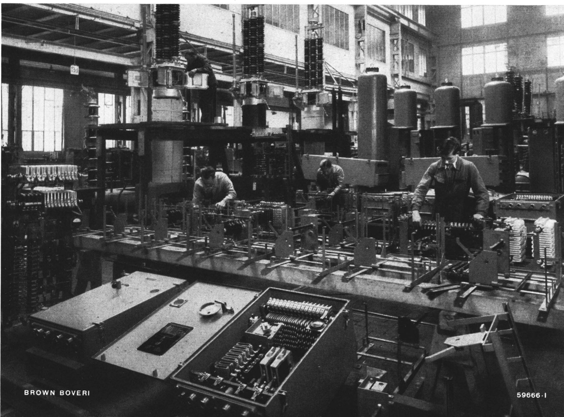
Fig. 177. — View of the workshops where our d. c. marine starters for motors up to 70 H.P. are produced in series and kept in stock without resistance elements and coils, to enable them to be supplied at short notice.
