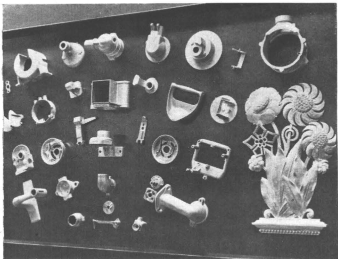
P ANEL illustrating possibilities of production of small castings of varying intricacies of design in aluminium alloys.
