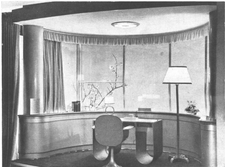
C URVED bay window and accessory furniture. The metalwork here is in anodized and dyed aluminium, the windows, desk top, handles and armrests of chair being in Perspex.
