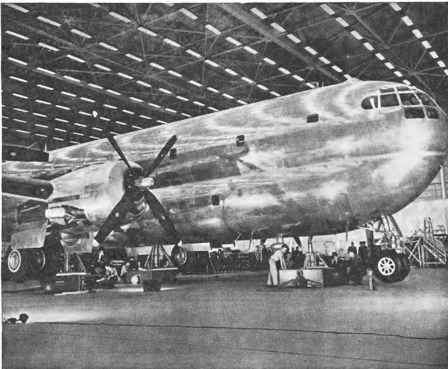
FIG. 4.—Weighing the C-97 (Stratocruiser). The neatness of this portable equipment for the weighing of such a large aeroplane is notable and may be studied in connexion with the article on pp. 250-253. It will be noted that the scales incorporate jacks, and that each unit is fitted with castors and handles for transport
