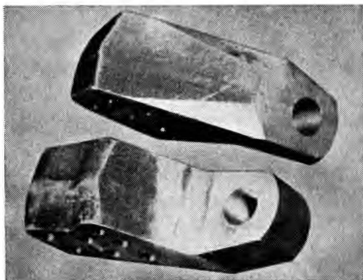
FIG. 3.—These forgings have some surfaces hyper-milled and some faced with conventional cutters, the former being much smoother than the latter.
