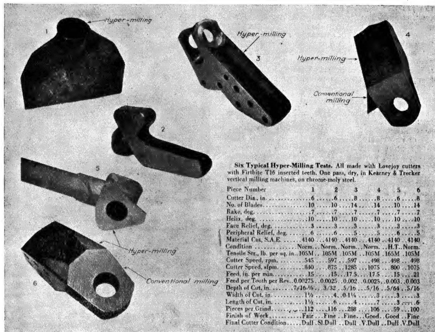
FIG. 4.—Six specimens tested, with detailed data on each.
