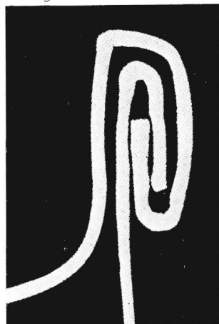
5. Seam very badly sprung causing loosening of seam and bulging of countersink.
