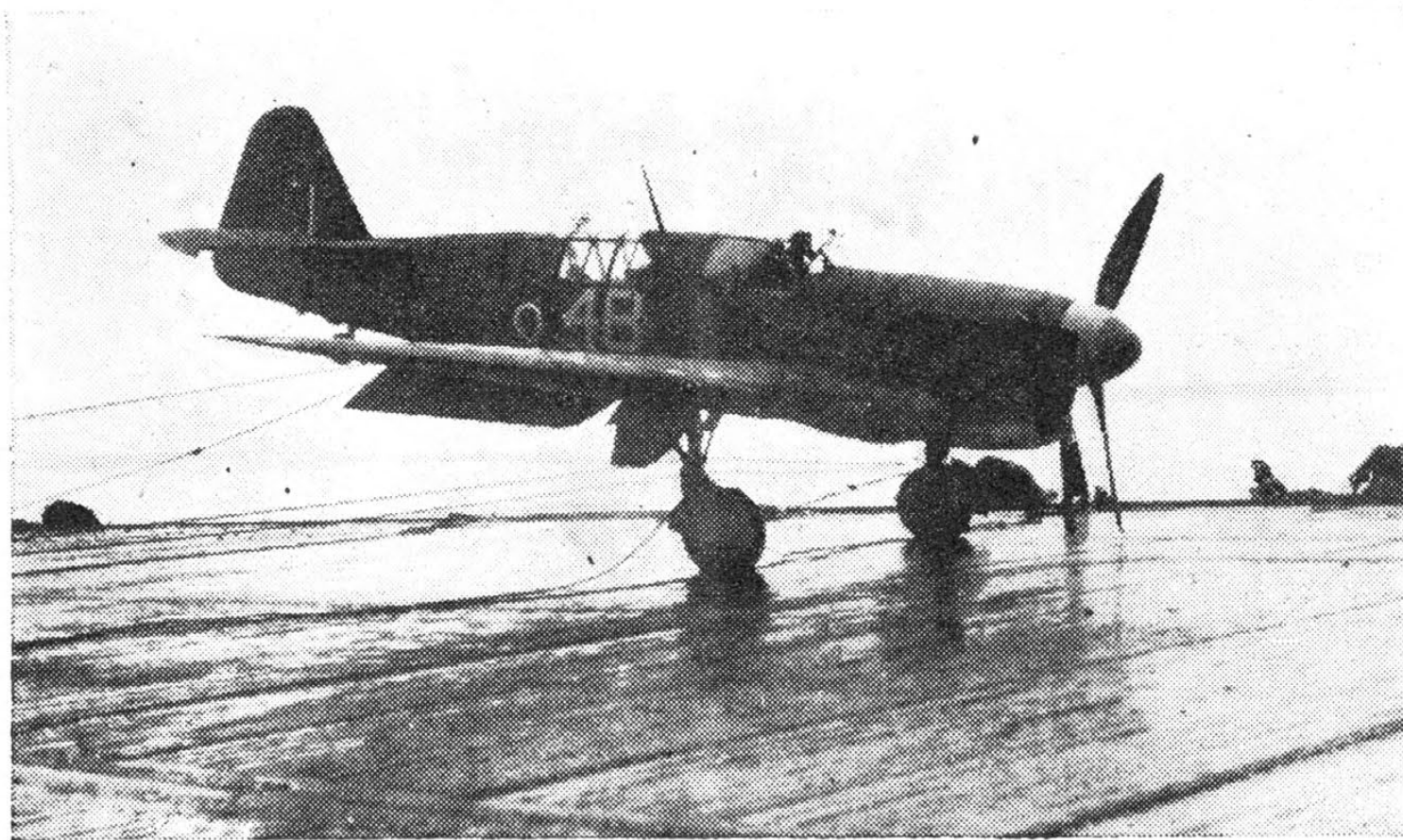
CARRYING ALL BEFORE HIM : A Firefly pilot, undergoing training on the escort carrier H.M.S. Empress , trips up slightly in landing-on. Observe the tip of one airscrew blade, bending as it hits the deck.
