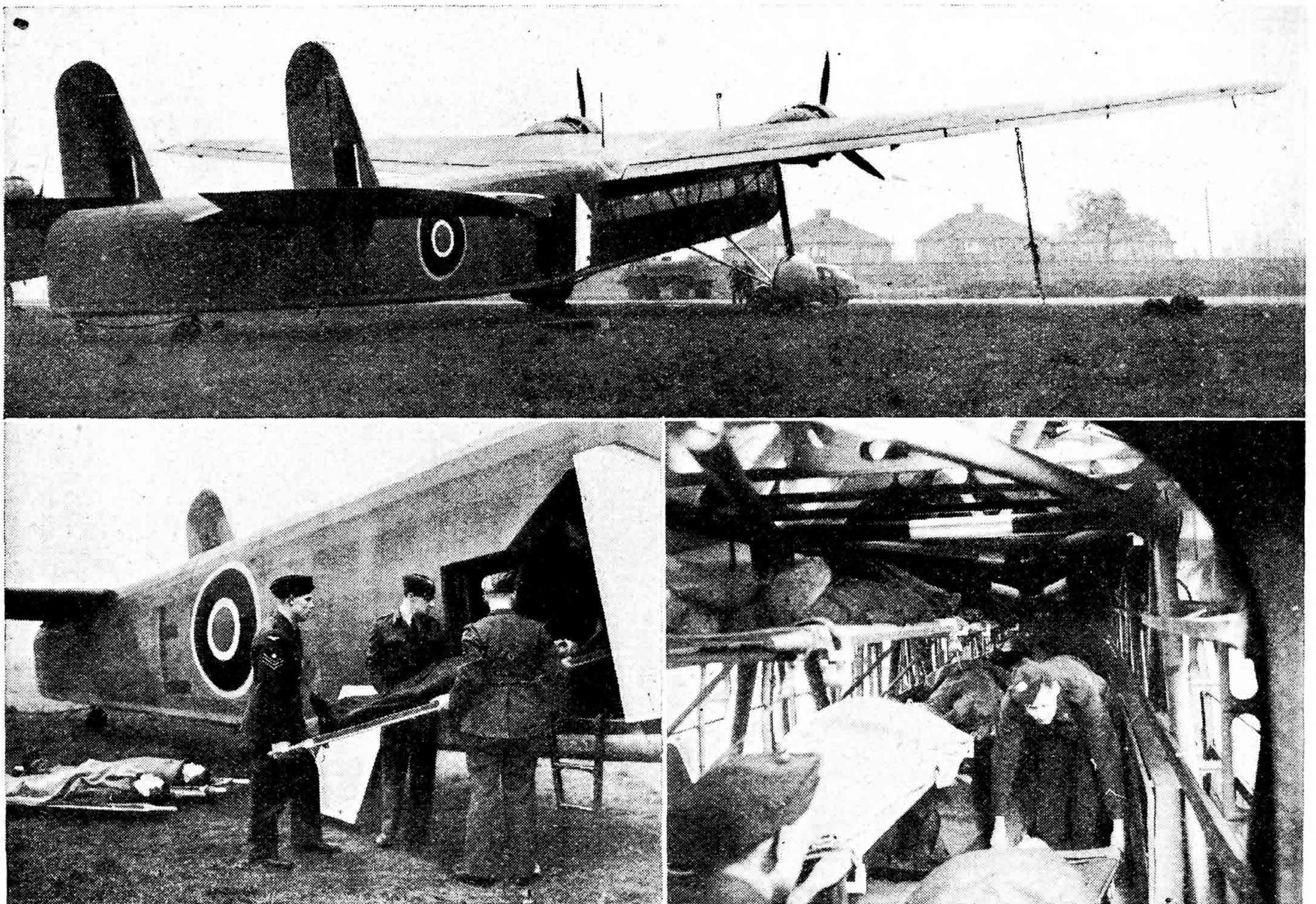
BLOOD WAGONS —I.—The first pictures to be released of the Handley Page Harrow in use as an air ambulance. Nose and tail turrets have been removed and faired in. (Bottom left) In order to facilitate the loading of the stretchers, the door in the starboard side has been enlarged and modified in shape. (Bottom right) The spacious fuselage of this ex-bomber transport is well suited to carry the patients with the maximum of comfort, at the same time leaving plenty of room for the medical personnel to attend to their charges whilst in flight. The nick-name "Blood Wagon" is R.A.F. slang.
