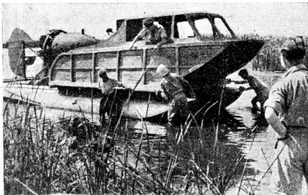
THE RETRIEVER. —A "home-made" hydroplane which forms part of the R.A.F.'s "Sea-Air" rescue service on the lakes of the Nile Delta. It consists of a cabin mounted on seaplane floats, is driven by an aero-motor and propeller mounted in the stern, and is steered by an aeroplane rudder. Each of the floats also has a water rudder. The craft can make a good 15 knots.
