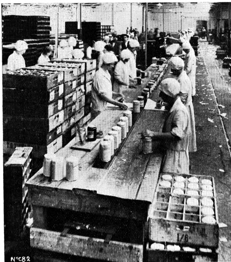
Fig. 4.—View from the delivery terminal of conveyor for assisting the operations of labelling, capping, wrapping and packing jars of jam in a preserve factory.
