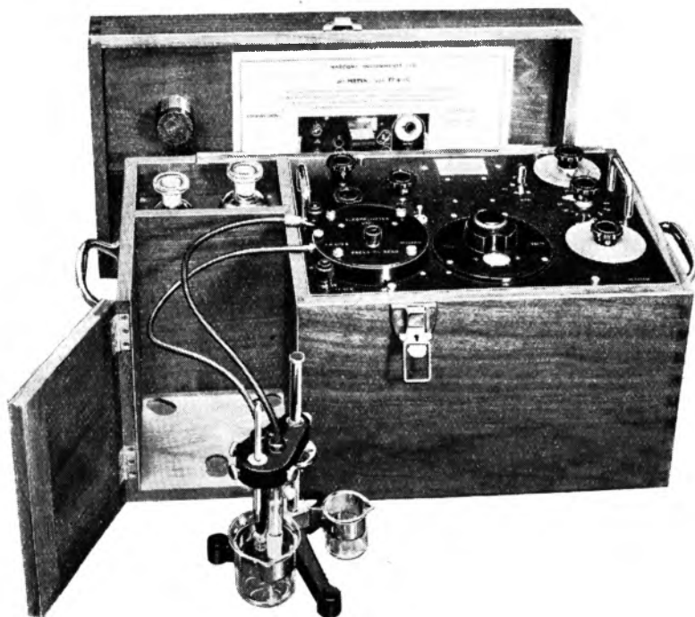
For practical purposes in works, pH meters based on electronic principles are available. The picture shows a pH meter operated from internal dry batteries.
