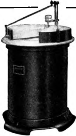
Above: Vertical Type Electric Furnace, most suited for hardening components which are prone to distortion if laid on a furnace hearth.
