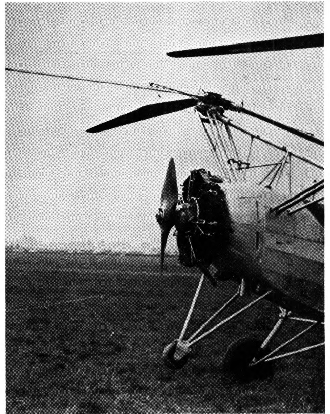
FIG. 20 SHOWING PROPELLER-TYPE BLOWER FOR COOLING ENGINE IN HOVERING FLIGHT
