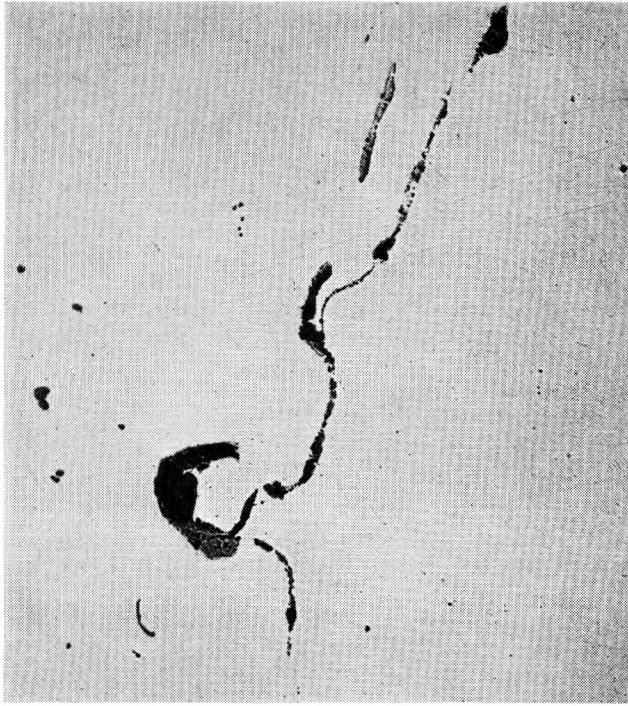
FIG. 17 FISSURES AND VOIDS IN THE ADDED METAL NEAR THE FUSION ZONE PARTIALLY FILLED WITH OXIDES. \times 100
