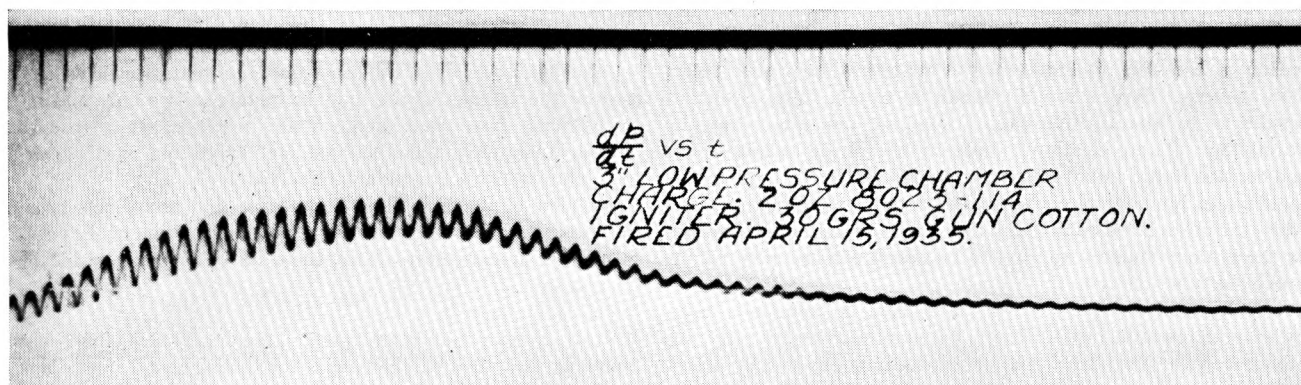
FIG. 14 SHOWING dp/dt FOR A CLOSED CHAMBER
