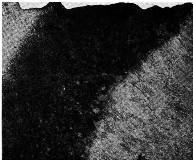
FIG. 15 VOIDS IN THE WELD METAL WHICH WERE ALSO THE STARTING POINT OF CRACKS. SECTION ETCHED WITH 1 PER CENT NITAL. \times 25
