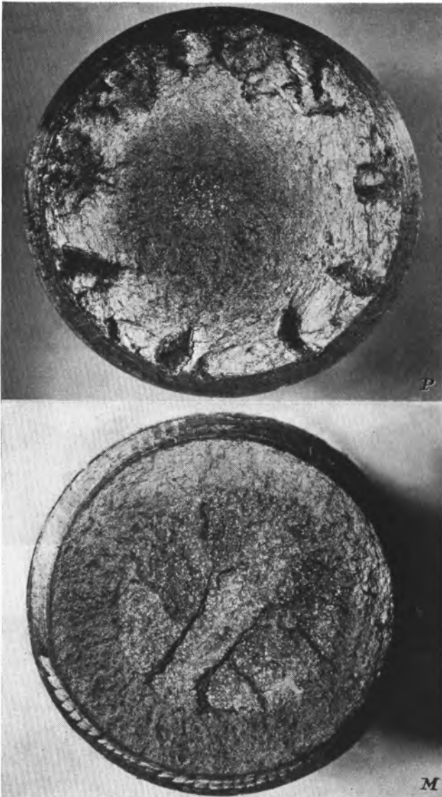
FIG. 14 FRACTURE SURFACES OF NOTCHED BARS (Bar P shows fracture of a notched bar in pure torsion; bar M tested with combined tension and torsion.)
