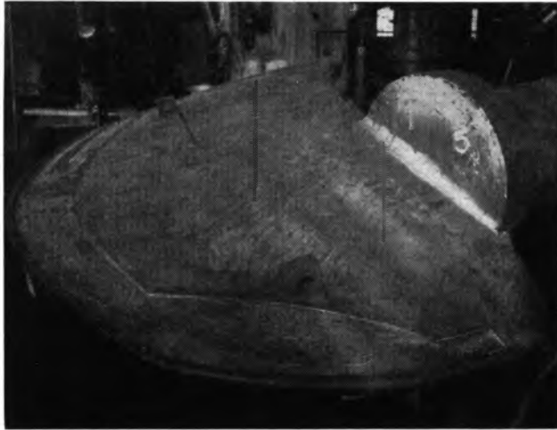
FIG. 2 TURBINE-RUNNER BLADE BEFORE BEING PREWELDED
