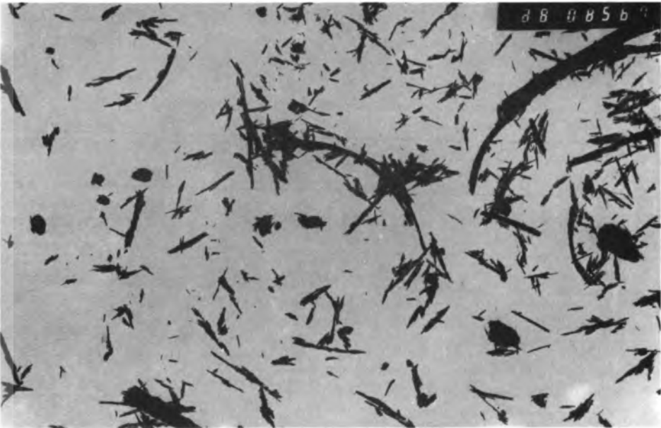
Fig. 2. Electron micrograph of the chrysotile heated at 600°C.
