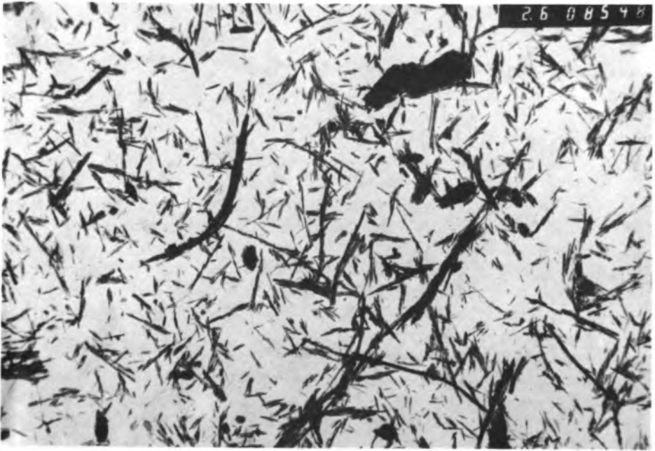
Fig. 1. Electron micrograph of the chrysotile unheated.
