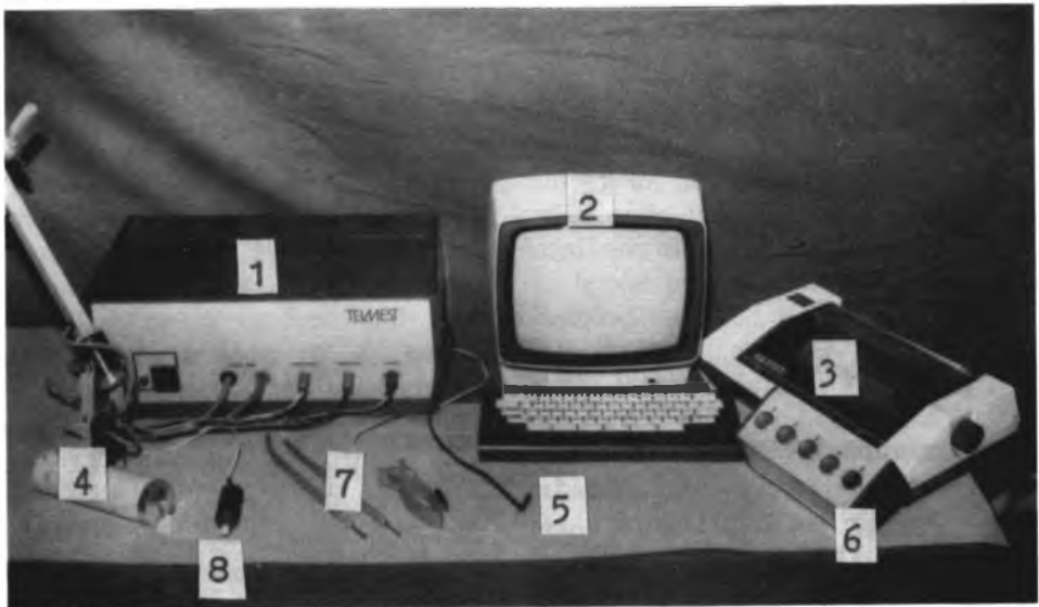
Fig. 1. TELMEST: 1) Main console containing computer and decisive module systems. 2) Video display unit with keyboard. 3) Printer. 4) Movable applicator of vibration. 5) Thermistor probe of actual temperature. 6) Applicator of constant temperature stimuli. 7) Applicators of current stimuli. 8) Switch for proband's of stimulus perception.
